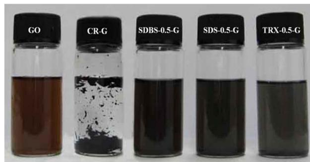
Fig. 17 Digital photographs of water dispersion of pure GO, CR-G, SDBS-0.5-G, SDS-0.5-G and TRX-0.5-G. Reproduced with permission.<sup>72</sup> Copyright Elsevier 2013.
