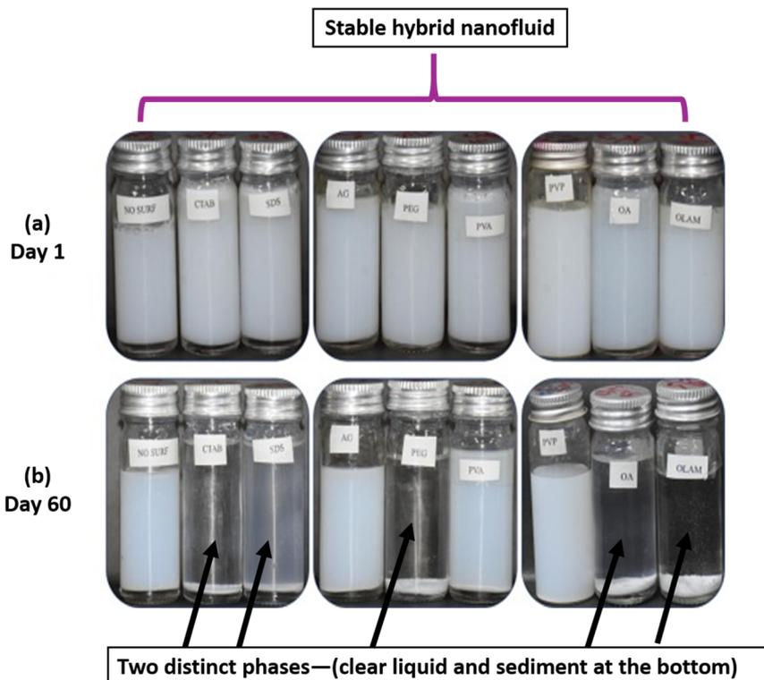
Fig. 7 Comparison of the visual sedimentation evaluation of hybrid nanofluids at (a) day 1 and (b) day 60 using the visual sedimentation method. Reproduced with permission.<sup>41</sup> Copyright Elsevier 2003.
