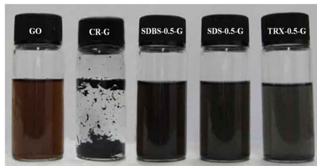
Fig. 17 Digital photographs of water dispersion of pure GO, CR-G, SDBS-0.5-G, SDS-0.5-G and TRX-0.5-G. Reproduced with permission. 72 Copyright Elsevier 2013.
