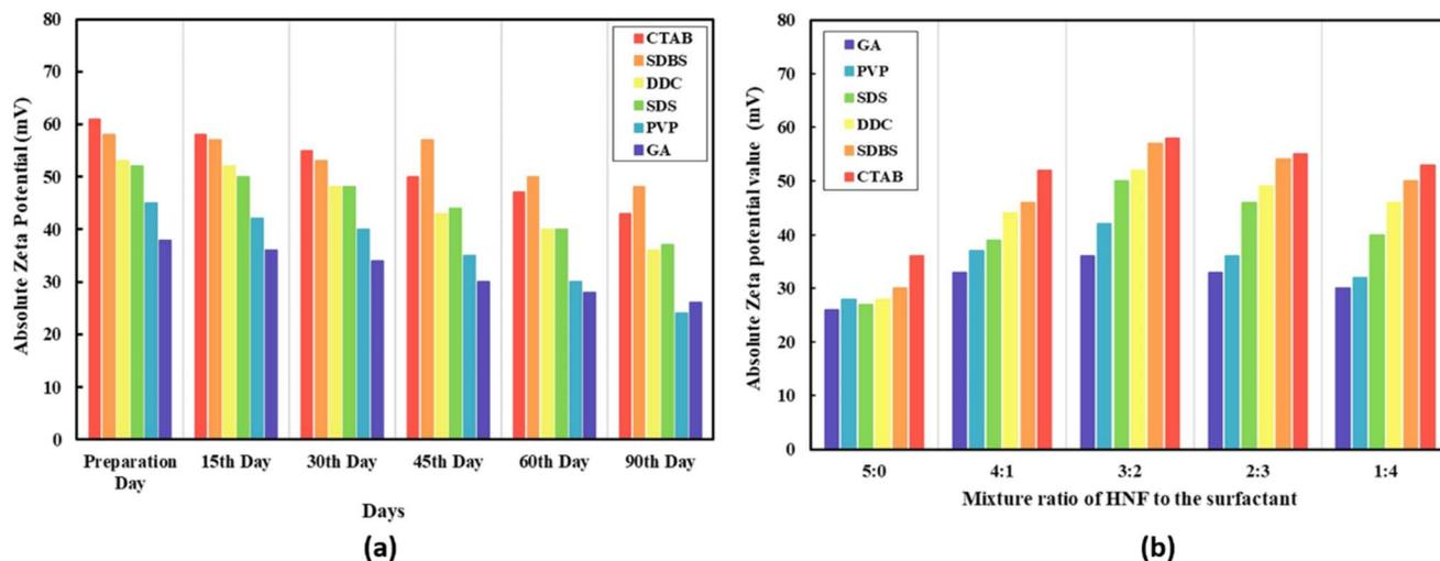
Fig. 9 (a) Effect of different surfactants on the absolute zeta potential of the prepared ( $\text{CeO}_2 + \text{MWCNTs}$  (80 : 20)) water-based hybrid nanofluid over 90 days from the preparation. (b) Effect of the mixture ratio of volume concentration to the surfactant on the stability of HNF ( $\text{CeO}_2 + \text{MWCNTs}$  (80 : 20)) on the 15th day of preparation. Reproduced with permission.<sup>45</sup> Copyright Elsevier 2021.
