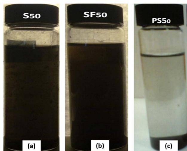
Fig. 15 Visual observation test for the functionalized MWCNT hybrid nanofluid: (a) S 50, (b) SF50 and (c) hybrid nanofluid with unfunctionalized MWCNTs (PS 50). Reproduced with permission.<sup>70</sup> Copyright Elsevier 2013.
