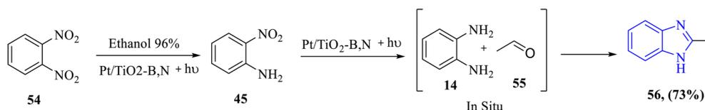
Scheme 15 One-pot synthesis of benzimidazole **56** *via* photocatalytic reduction of dinitrobenzene (**54**) to *O*-phenylenediamine **14** followed by condensation with aldehyde **55** using a Pt/TiO<sub>2</sub>-B,N catalyst in ethanol.
