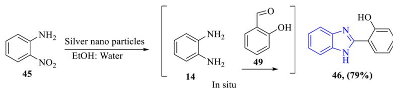
**Scheme 12** Green one-pot synthesis of benzimidazole **46** via silver nanoparticle-catalyzed reduction of 2-nitroaniline **45** to *O*-phenylenediamine **14**, followed by reaction with aldehyde **49**.
