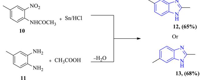
Fig. 3 The first schemes used for benzimidazole synthesis.
