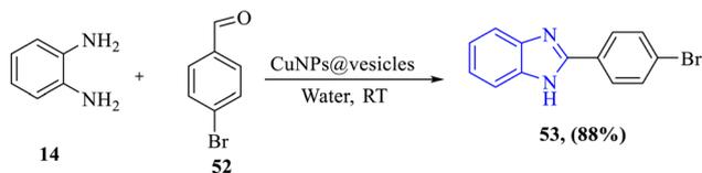
Scheme 14 One-pot synthesis of 2-substituted benzimidazole **53** using CuNPs@vesicle nanoreactors, converting 2-nitroaniline into *O*-phenylenediamine **14**, followed by reaction with substituted aldehydes **52** in an aqueous medium.
