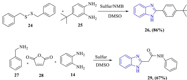
**Scheme 5** Sulfur-catalyzed synthesis of benzimidazole **26** from 1,2-dibenzyl disulfane **24** and *O*-phenylenediamine derivative **25** in NMP/DMSO at 100 °C. One-pot, multi-component synthesis of benzimidazole **29** from benzylamine **27**, maleic anhydride **28**, and *O*-phenylenediamine **14** using a sulfur catalyst and DMSO as an oxidant.
