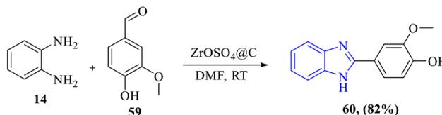
Scheme 17 Room-temperature light-assisted synthesis of benzimidazole **60** from *O*-phenylenediamine **14** and aldehyde **59** catalyzed using solid-state ZrOSO<sub>4</sub>@C acid.
