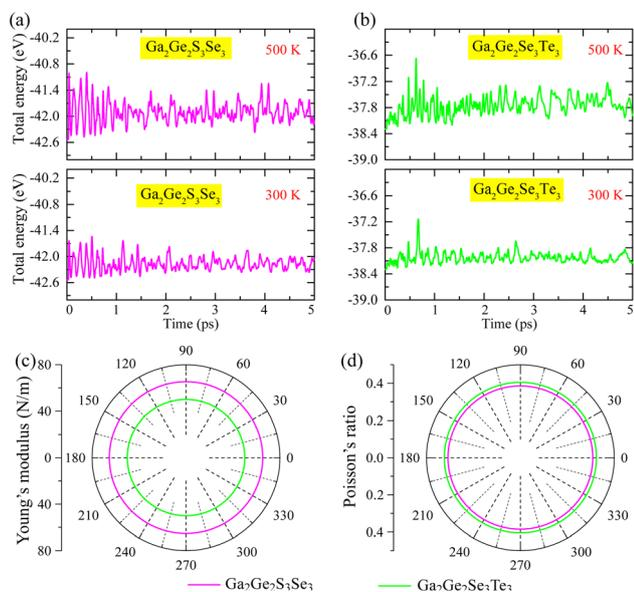
Fig. 2 (a and b) Total energy variation of  $\text{Ga}_2\text{Ge}_2\text{S}_3\text{Se}_3$  and  $\text{Ga}_2\text{Ge}_2\text{Se}_3\text{Te}_3$  monolayers at 300 K and 500 K; angular functions of (c) Young's modulus and (d) Poisson's ratio of  $\text{Ga}_2\text{Ge}_2\text{S}_3\text{Se}_3$  (pink circles) and  $\text{Ga}_2\text{Ge}_2\text{Se}_3\text{Te}_3$  (green circles) monolayers.
