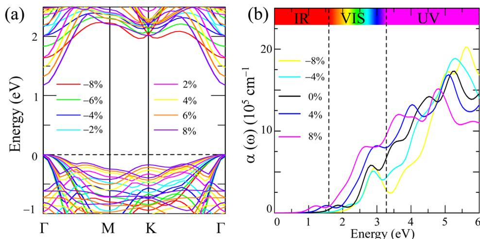
Fig. 6 (a) Impact of strain on the band structure and (b) the light absorption rate of the Ga<sub>2</sub>Ge<sub>2</sub>S<sub>3</sub>Se<sub>3</sub> monolayer.
