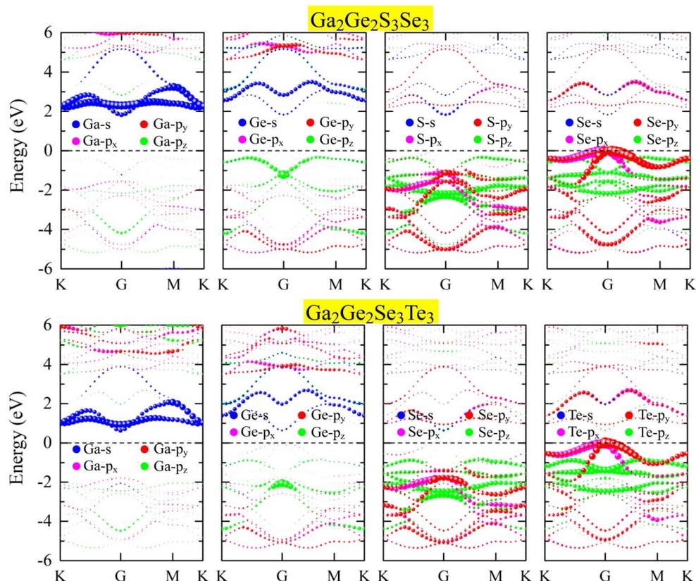
Fig. 4 Orbital-projected band structures of  $\text{Ga}_2\text{Ge}_2\text{S}_3\text{Se}_3$  and  $\text{Ga}_2\text{Ge}_2\text{Se}_3\text{Te}_3$  monolayers.
