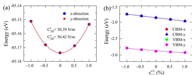
Fig. 8 (a) Total energy  $E_{\text{total}}$  and (b) band edge energy  $E_{\text{edge}}$  as functions of uniaxial strains  $\varepsilon_{\text{uni}}$  applied on the  $\text{Ga}_2\text{Ge}_2\text{S}_3\text{Se}_3$  monolayer.
