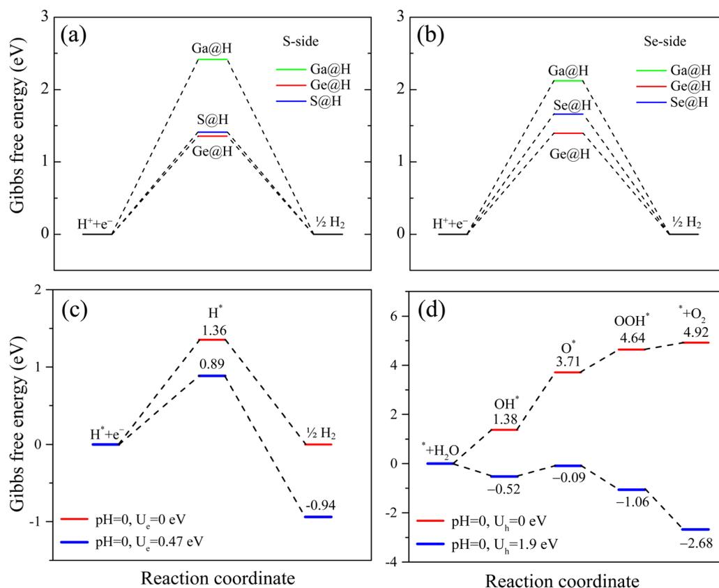
Fig. 7 (a and b) Gibbs free energy change as hydrogen atom is connected to the Ga, Se, or Ge atoms on the S-side and Se-side of in  $\text{Ga}_2\text{Ge}_2\text{S}_3\text{Se}_3$  monolayer; (c and d) photocatalytic reaction steps of HER and OER half-reactions.
