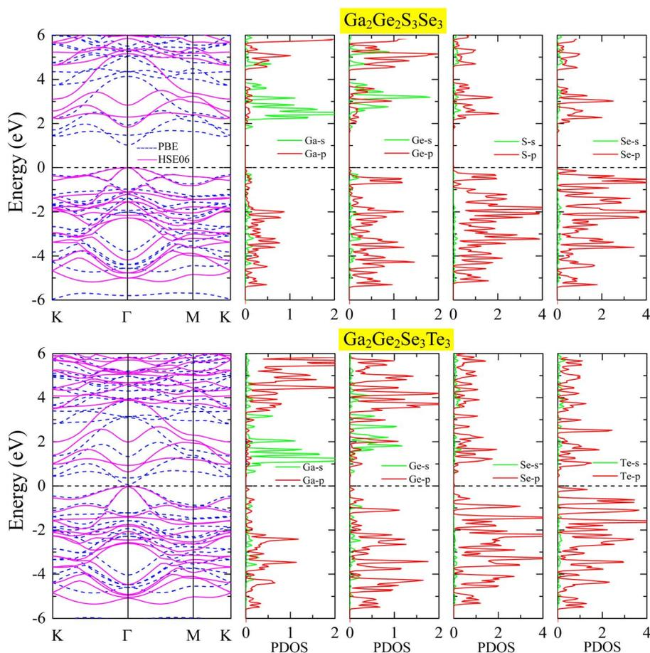
Fig. 3 Electronic band structures and projected density of states (PDOS) of  $\text{Ga}_2\text{Ge}_2\text{S}_3\text{Se}_3$  and  $\text{Ga}_2\text{Ge}_2\text{Se}_3\text{Te}_3$  monolayers. The band structures were calculated using PBE functional (dash blue lines) and HSE06 hybrid functional (solid pink lines).
