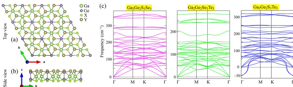
Fig. 1 Optimized atomic structure of  $\text{Ga}_2\text{Ge}_2\text{X}_3\text{Y}_3$  ( $\text{X}/\text{Y} = \text{S}, \text{Se}, \text{Te}; \text{X} \neq \text{Y}$ ) monolayers shown in (a) top view and (b) site view together with (c) their phonon dispersions.
