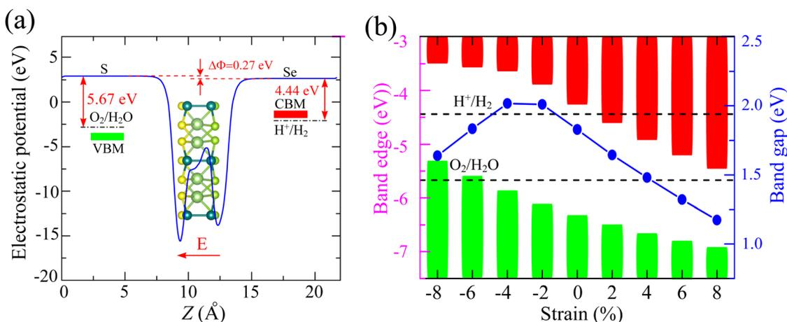
Fig. 5 (a) Electrostatic potential with intrinsic electric field (red arrow) of Ga<sub>2</sub>Ge<sub>2</sub>S<sub>3</sub>Se<sub>3</sub> monolayer and (b) the variation of bandgap and band edge alignment relative to the redox potential of water splitting reaction.
