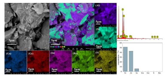
Fig. 4 SEM-EDS analysis of gasification slag obtained at 1500 °C.
