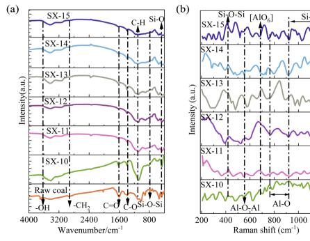
Fig. 3 FTIR (a) and Raman (b) spectra of coal and different slags.
