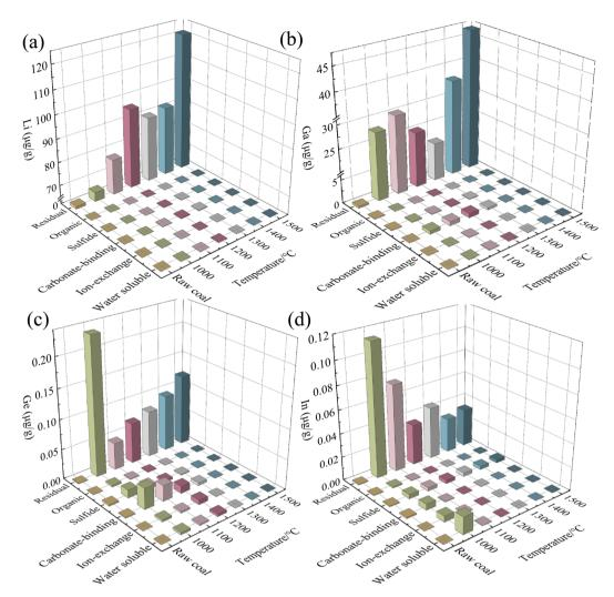
Fig. 5 Occurrence form and enrichment content of the critical metal elements: lithium (a), gallium (b), germanium (c), and indium (d).
