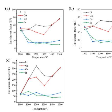
Enrichment factor of different critical metal elements and Al<sub>2</sub>O<sub>3</sub> (a), SiO<sub>2</sub> (b), and SO<sub>3</sub> (c).
