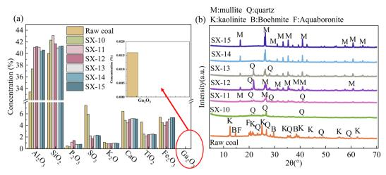
Fig. 2 XRF (a) with the inset showing a magnified view of the area marked by the red circle, and XRD (b) spectra of coal and different slags.
