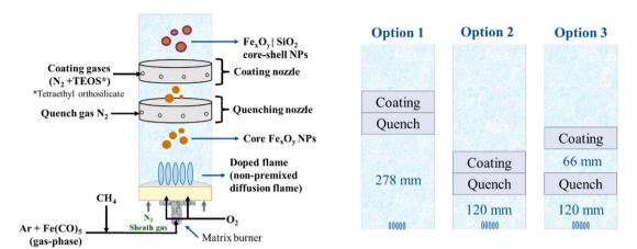
Fig. 1 Reactor setup (left) and different nozzle configurations with spacings between the burner-nozzles marked (right).
