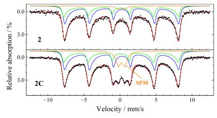
Fig. 6 Mössbauer spectra recorded at 300 K, showing contributions of the iron ions on A- (green), B-sites (blue), and superparamagnetic nanoparticles (orange). Due to the stronger superposition and the deformation of the spectral structure by superparamagnetic relaxation, B-site contributions of  $Fe^{2+}$  and  $Fe^{3+}$  were not reproduced individually. Refer to online publication for colors.
