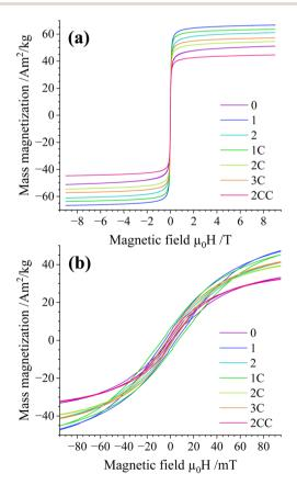
Fig. 7 (a) M(H) magnetization curves recorded at 300 K and (b) zoomin of (a). Magnetization values are normalized to the total sample mass. Refer to online publication for colors.
