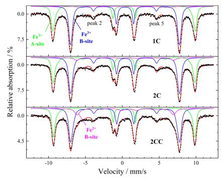
Fig. 5 Mössbauer spectra recorded at 5 K in a magnetic field of 8 T applied parallel to  $\gamma$ -ray propagation direction, showing contributions of Asite (green), B-site Fe<sup>3+</sup> (blue), and B-site Fe<sup>2+</sup> (pink). Refer to online publication for colors.
