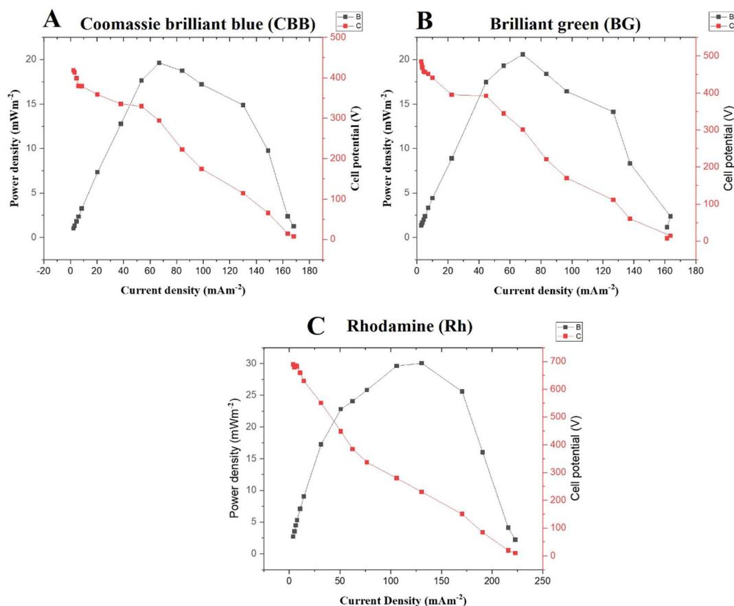
Fig. 5 Comparison of the polarization curve for PMA-MFC1-3 enriched with diatomite: (A) PMA-MFC 1 (diatomite–Coomassie brilliant blue- $\text{Fe}_3\text{O}_4$ ); (B) PMA-MFC 2 (diatomite–brilliant green- $\text{TiO}_2$ ) and (C) PMA-MFC 3 (diatomite–rhodamine- $\text{TiO}_2$ ).
