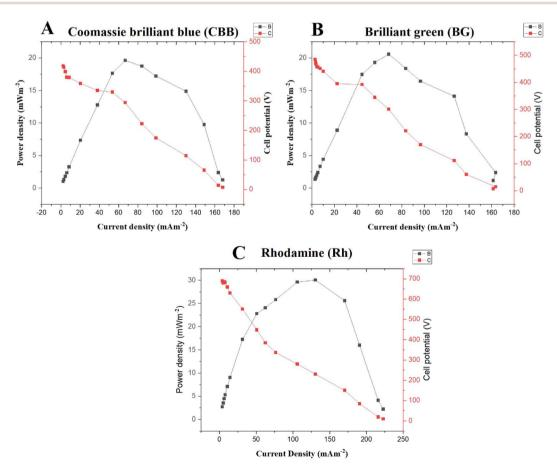
Fig. 5 Comparison of the polarization curve for PMA-MFC1-3 enriched with diatomite: (A) PMA-MFC 1 (diatomite—Coomassie brilliant blue—Fe<sub>3</sub>O<sub>4</sub>); (B) PMA-MFC 2 (diatomite—brilliant green—TiO<sub>2</sub>) and (C) PMA-MFC 3 (diatomite—rhodamine—TiO<sub>2</sub>).
