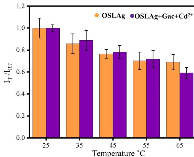
Fig. 9 Fluorescence intensities of OSLAg and OSLAgGacCd<sup>2+</sup> at various temperatures with respect to the room temperature.
