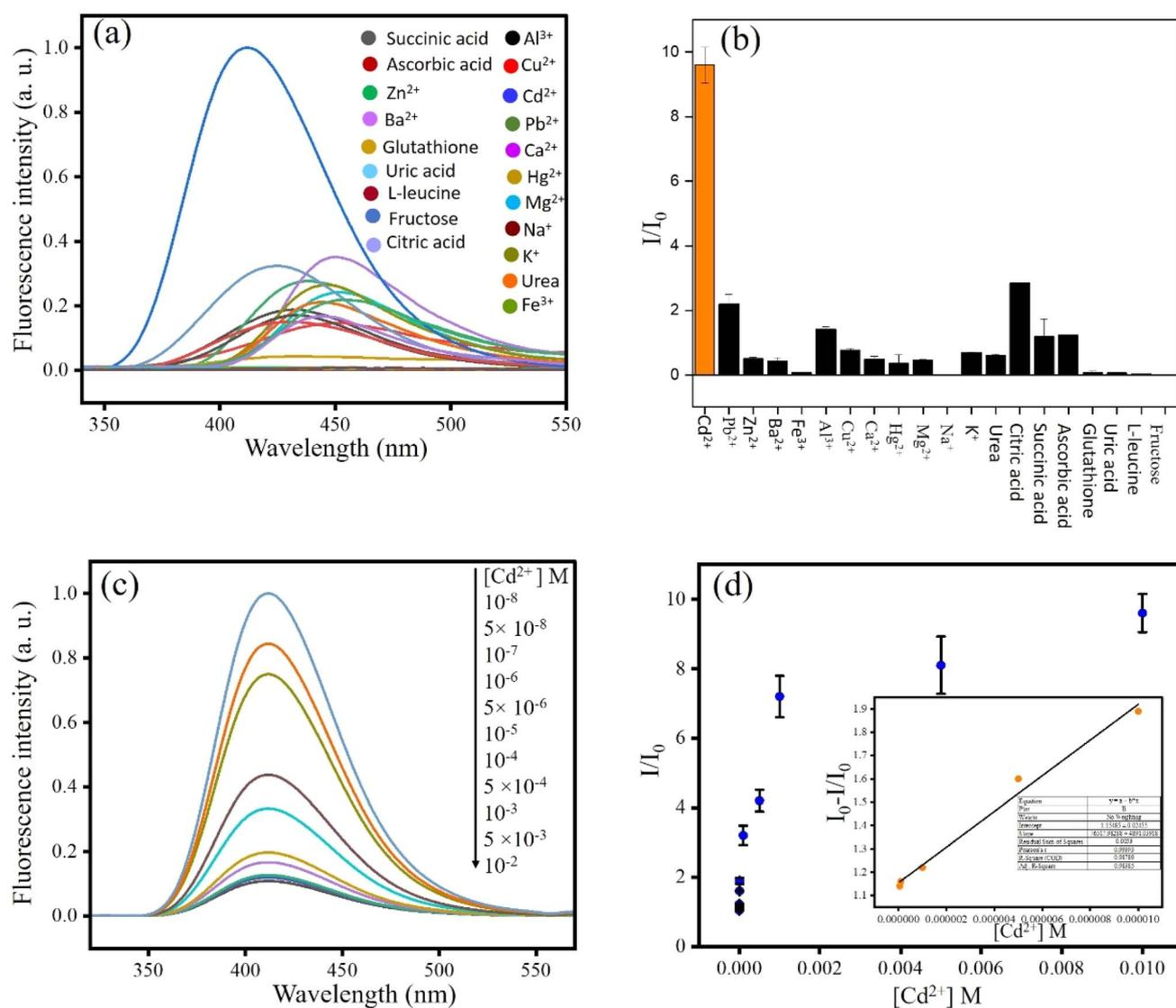
Fig. 6 (a) Fluorescence spectra of OSLAg + OGAc in the presence of various metal ions. (b) Bar diagram of  $I/I_0$  for different metal ions. (c) Fluorescence spectra of OSLAg + OGAc with different  $[\text{Cd}^{2+}]$ ; (d) plot of  $I/I_0$  vs.  $[\text{Cd}^{2+}]$ ; inset shows the linear detection range for  $\text{Cd}^{2+}$  detection.
