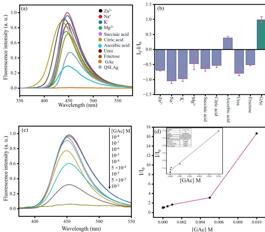
Fig. 4 (a) Emission spectra of OSLAg in the presence of different metal ions. (b) Bar diagram of  $I_0 - III_0$  for different metal ions. (c) Emission spectra of OSLAg with different [GAc]. (d) Plot of  $I/I_0$  vs. [GAc]; inset shows the linear detection range for GAc detection.
