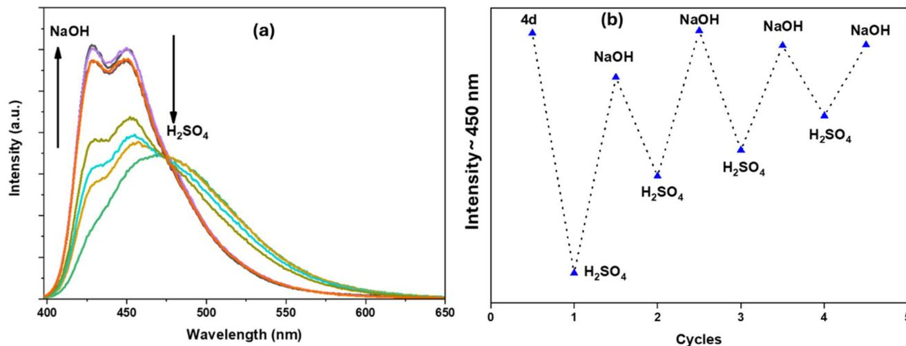
Fig. 7 (a) Emission spectra of **4d** ( $1 \times 10^{-6}$  M in THF) in different acidic and basic solutions (excitation wavelength: 365 nm). (b) Change of the emission intensity at  $\sim 450$  nm upon adding  $\text{H}_2\text{SO}_4$  and NaOH (excitation wavelength: 365 nm).
