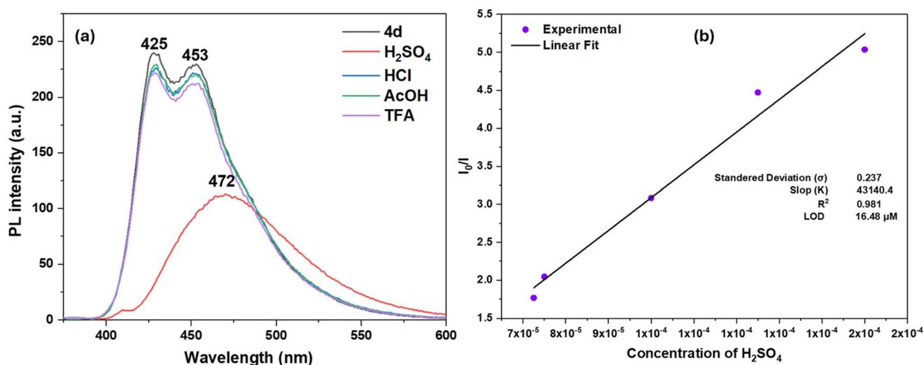
Fig. 6 (a) Emission spectra of **4d** ( $1 \times 10^{-6}$  M in THF) in various acid solutions (excitation wavelength: 365 nm). (b) Linear correlation of  $I_0/I$  vs. the concentrations of H<sub>2</sub>SO<sub>4</sub> in the range  $0.5 \times 10^{-5}$  to  $1.75 \times 10^{-4}$  M.
