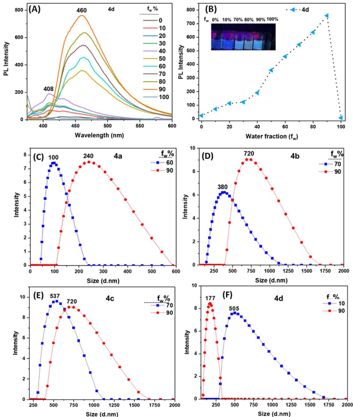
Fig. 2 (A) Emission spectra of 4d in THF/water mixtures (0–100%); (B) plot of maximum emission intensity of 4d versus water fraction; (C–F) dynamic light-scattering (DLS) spectra of 4a–d in THF/water, at specific  $f_w$  ratio.
