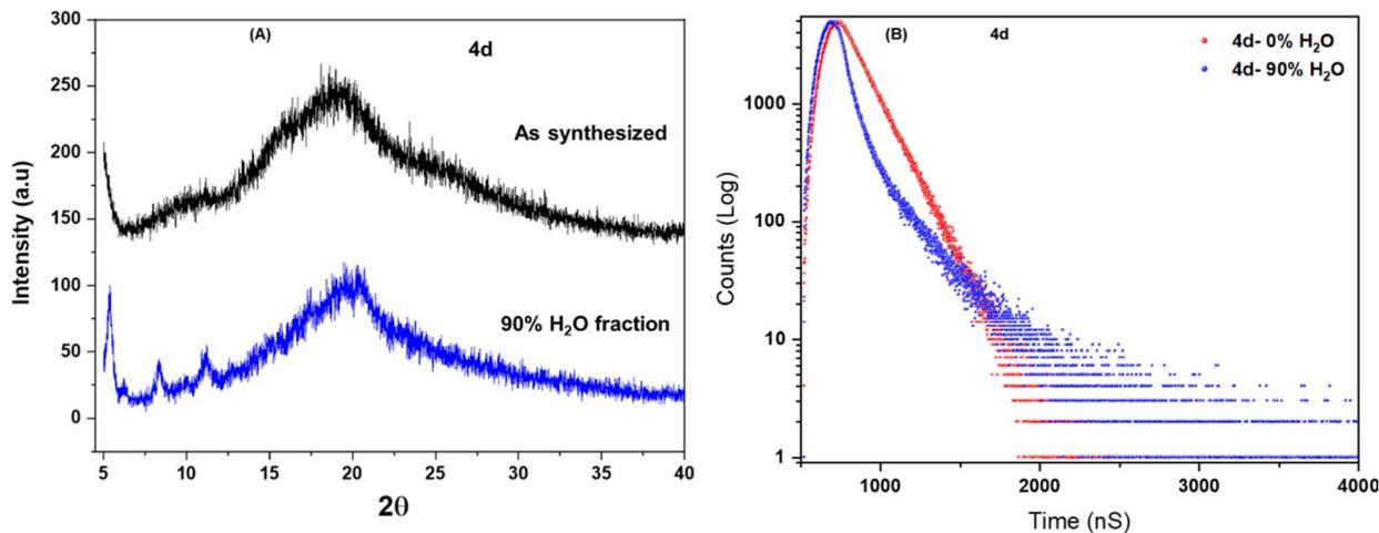
Fig. 3 (A) Powder XRD pattern of the synthesized (black graph) and THF/water,  $f_w$  90% (blue graph) of **4d** and (B) fluorescence lifetime decay profiles of **4d** in THF/water,  $f_w$  %: 0 (red graph) and 90 (blue graph).
