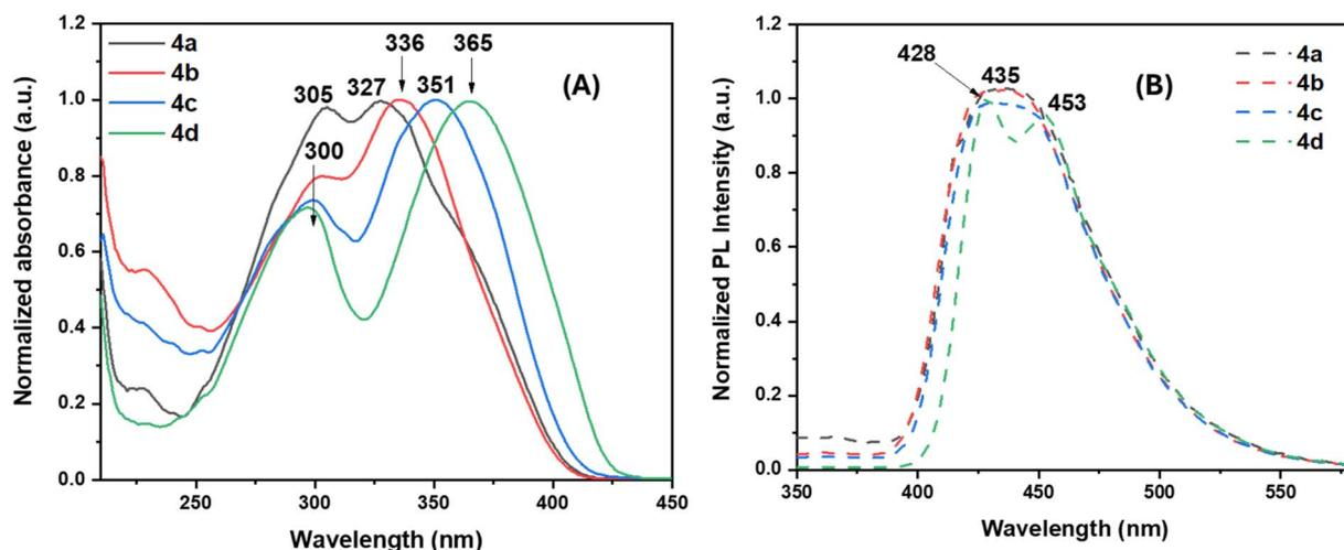
Fig. 1 Normalized UV/vis absorption (A) ( $C_M = 10^{-6}$  M solid lines) and emission (B) ( $C_M = 10^{-7}$  M dashed lines) spectra of compounds **4a–d** recorded in THF (absorption maxima were used as the excitation wavelengths).
