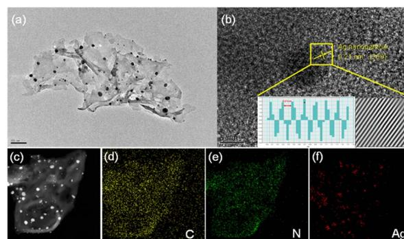
Fig. 1 (a) TEM image, (b) high-resolution image, and (c–f) EDS mapping of C, N and Ag elements of CNAg-30.
