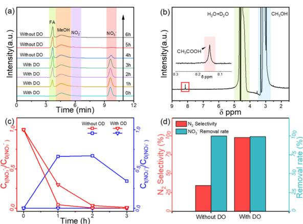
Fig. 5 (a) Ion chromatogram of photocatalysis with and without dissolved  $O_2$ . (b)  $^1H$  NMR spectroscopy of photocatalytic production with dissolved  $O_2$ . (c) Evolution of  $NO_3^-$  and  $NO_2^-$  during photocatalysis with and without dissolved  $O_2$  and (d)  $NO_3^-$  removal rate and  $N_2$  selectivity after 3 h.
