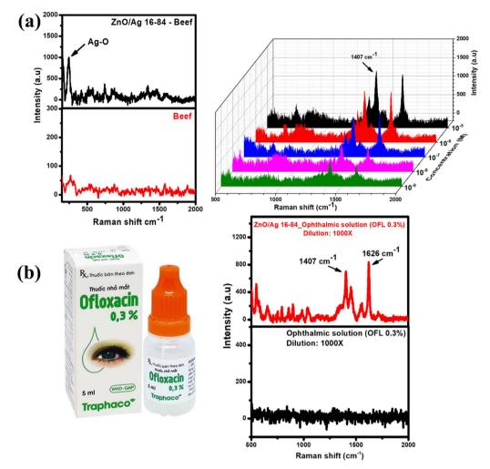
Fig. 8 (a) Raman spectra of beef sample (black line) on ZnO/Ag substrate in comparison to those of beef sample in the absence of ZnO/Ag (red line) (left); SERS spectra of OFL with different concentrations in real sample of beef on the ZnO/Ag SERS substrates (right); (b) 0.3 wt% OFL eye drop (left) and SERS spectra of 0.3 wt% OFL eye drop samples diluted 1000 times without and with the ZnO/Ag 16–84 SERS substrate (right).
