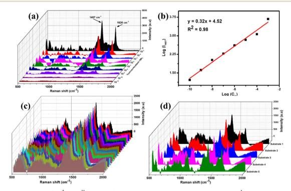
Fig. 4 (a) SERS spectra of OFL  $(10^{-3} \text{ to } 10^{-11} \text{ M})$  on ZnO/Ag. (b) Plot of the log of SERS intensity at 1407 cm<sup>-1</sup> against OFL concentration. (c) Uniformity and (d) reproducibility of SERS sensors for OFL  $(10^{-6} \text{ M})$  using the ZnO/Ag substrate (with 16 wt% of ZnO).
