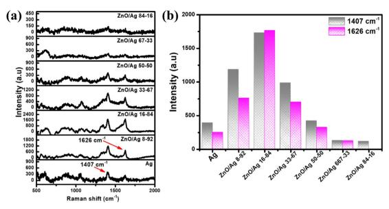
Fig. 3 (a) SERS spectra of OFL ( $10^{-5}$  M) on AgNPs, and ZnO/Ag nanocomposites with different ZnO contents. (b) SERS intensities of OFL ( $10^{-5}$  M) at 1407 and 1626 cm<sup>-1</sup> on AgNPs, and ZnO/Ag nanocomposites with different ZnO contents.
