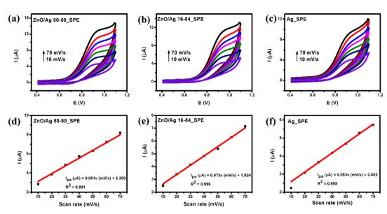
Fig. 6 (a-c) CVs responses of 100  $\mu$ M ofloxacin at the modified electrodes in 0.1 M PBS buffer at different scan rates, and (d-f) plots of the peak current (I) versus scan rate (V).
