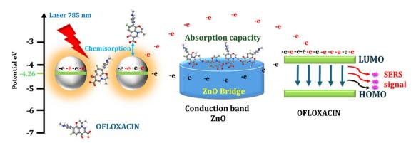
Fig. 7 Schematic proposed mechanism of charge transfer from ZnO/Ag to ofloxacin.
