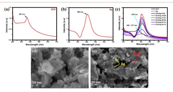
Fig. 1 UV-vis spectra of (a) ZnO nanosheets, (b) Ag NPs, and (c) pure Ag NPs, pure ZnO nanosheets, and ZnO/Ag nanocomposites with different ratios; SEM images of (d) ZnO nanosheets and (e) ZnO/Ag nanocomposite.
