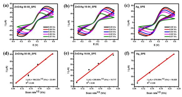
Fig. 5 CV curves recorded on ZnO/Ag 50–50\_SPE (a), ZnO/Ag 16–84\_SPE (b) and Ag\_SPE (c) in 0.1 M KCl containing 5 mM  $[Fe(CN)_6]^{3-}$   $[Fe(CN)_6]^{4-}$  with various scan rates from 0.01 to 0.05 V s<sup>-1</sup>, corresponding calibration plots of peak current response vs. square root of scan rate (d-f) with error bars.
