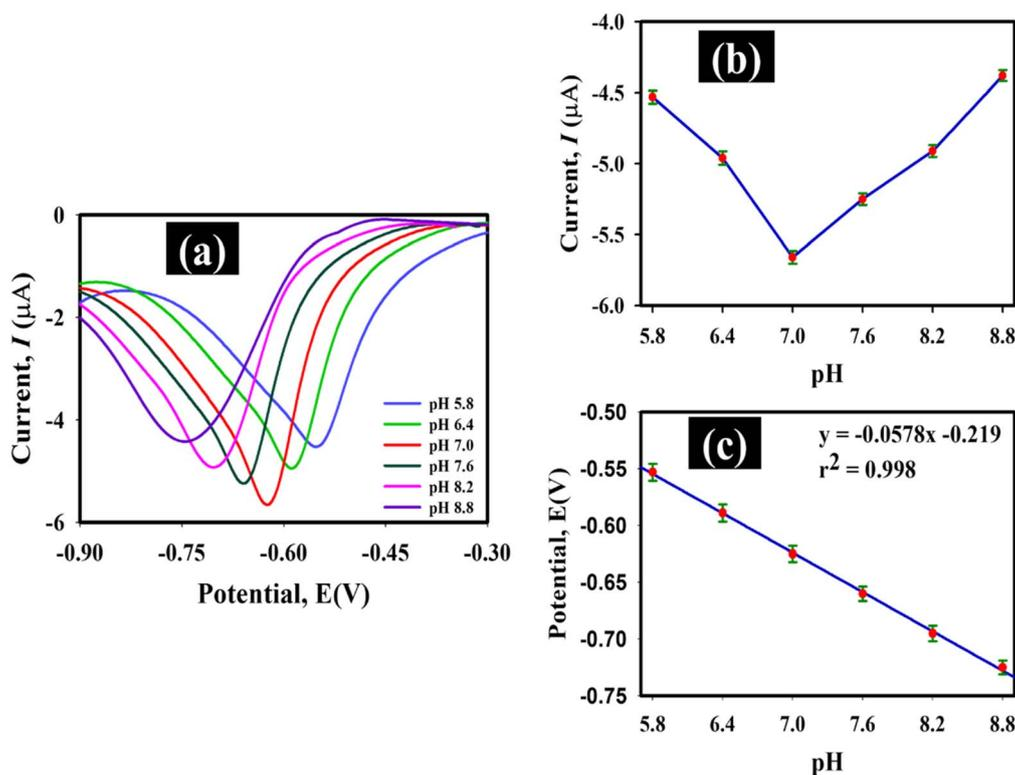
Fig. 7 (a) SWV responses of Au@rGO/CuO/GCE at various pH values (5.8–8.8) in 0.1 M PBS buffer with 10  $\mu M$  MP present, within a potential window of  $-0.3$  V to  $-0.9$  V. (b) The reduction current intensity vs. electrolyte pH. (c) The peak potential fluctuation as a function of the electrolyte pH.
