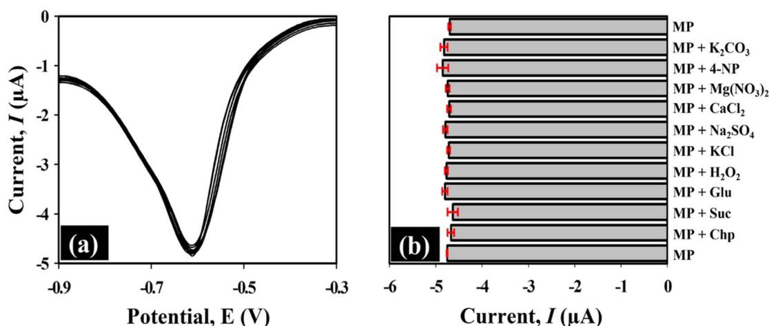
Fig. 10 (a) Selectivity test using SWV responses of Au@rGO/CuO/GCE to 10  $\mu$ M MP and the concentrations of inorganic interfering species:  $K_2CO_3$ ,  $Mg(NO_3)_2$ ,  $CaCl_2$ ,  $KCl$ , and  $Na_2SO_4$  along with organic species: 4-NP, glucose (Glu), sucrose (Suc), chlorpyrifos (Chp), and  $H_2O_2$  at 50  $\mu$ M. (b) Bar diagram of current response vs. MP and above-mentioned interfering species.
