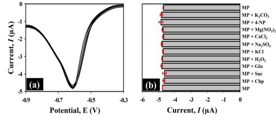
Fig. 10 (a) Selectivity test using SWV responses of Au@rGO/CuO/GCE to 10  $\mu$ M MP and the concentrations of inorganic interfering species:  $K_2CO_3$ ,  $Mg(NO_3)_2$ ,  $CaCl_2$ , KCl, and  $Na_2SO_4$  along with organic species: 4-NP, glucose (Glu), sucrose (Suc), chlorpyriphos (Chp), and  $H_2O_2$  at 50  $\mu$ M. (b) Bar diagram of current response vs. MP and above-mentioned interfering species.
