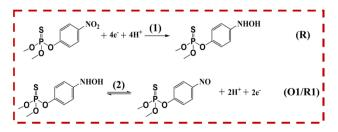
Scheme 1 Proposed electrochemical reaction mechanism.
