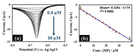
Fig. 9 (a) SWV response of Au@rGO/CuO/GCE in the potential window of -0.3 V to -0.9 V (with a 120 s accumulation time, pulse amplitude of 0.025 V, pulse increment of 0.004 V, and frequency of 15 Hz) as a function of MP concentration in 0.1 M PBS (pH = 7.0). Voltammograms without MP are displayed by the dashed line. (b) Calibration plot of reduction current vs. [MP].
