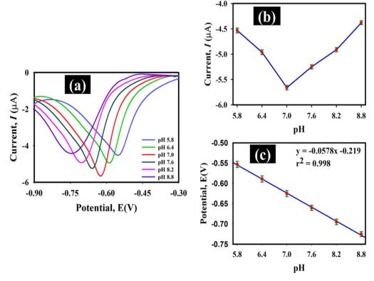
Fig. 7 (a) SWV responses of Au@rGO/CuO/GCE at various pH values (5.8–8.8) in 0.1 M PBS buffer with 10  $\mu$ m MP present, within a potential window of -0.3 V to -0.9 V. (b) The reduction current intensity vs. electrolyte pH. (c) The peak potential fluctuation as a function of the electrolyte pH.
