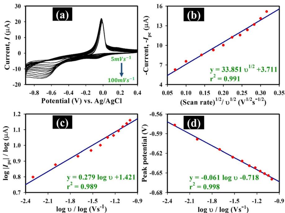
Fig. 8 (a) Voltammograms of Au@rGO/CuO/GCE at  $30 \mu\text{M}$  of MP in  $0.1 \text{ M PBS}$  (pH 7.0) obtained by varying the scan rate from  $5 \text{ mV s}^{-1}$  to  $100 \text{ mV s}^{-1}$ . (b) Correlation between the square root of the scan rate ( $\nu^{1/2}$ ) and cathodic peak current ( $I_{pc}$ ); (c) correlation between  $\log(I_{pc})$  and  $\log$  scan rate ( $\nu$ ); and (d) linear relationship between cathodic peak potential ( $E_p$ ) and  $\log \nu$ .
