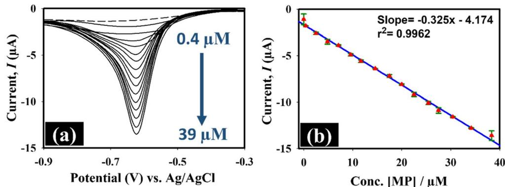
Fig. 9 (a) SWV response of Au@rGO/CuO/GCE in the potential window of  $-0.3$  V to  $-0.9$  V (with a 120 s accumulation time, pulse amplitude of 0.025 V, pulse increment of 0.004 V, and frequency of 15 Hz) as a function of MP concentration in 0.1 M PBS (pH = 7.0). Voltammograms without MP are displayed by the dashed line. (b) Calibration plot of reduction current vs. [MP].
