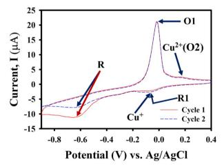
Fig. 5 Cyclic voltammograms of 2 consecutive cycles at a scan rate of 50 mV s $^{-1}$  for 30  $\mu$ m MP in 0.1 M PBS at pH = 7.0, starting from the potential of 0.4 V.
