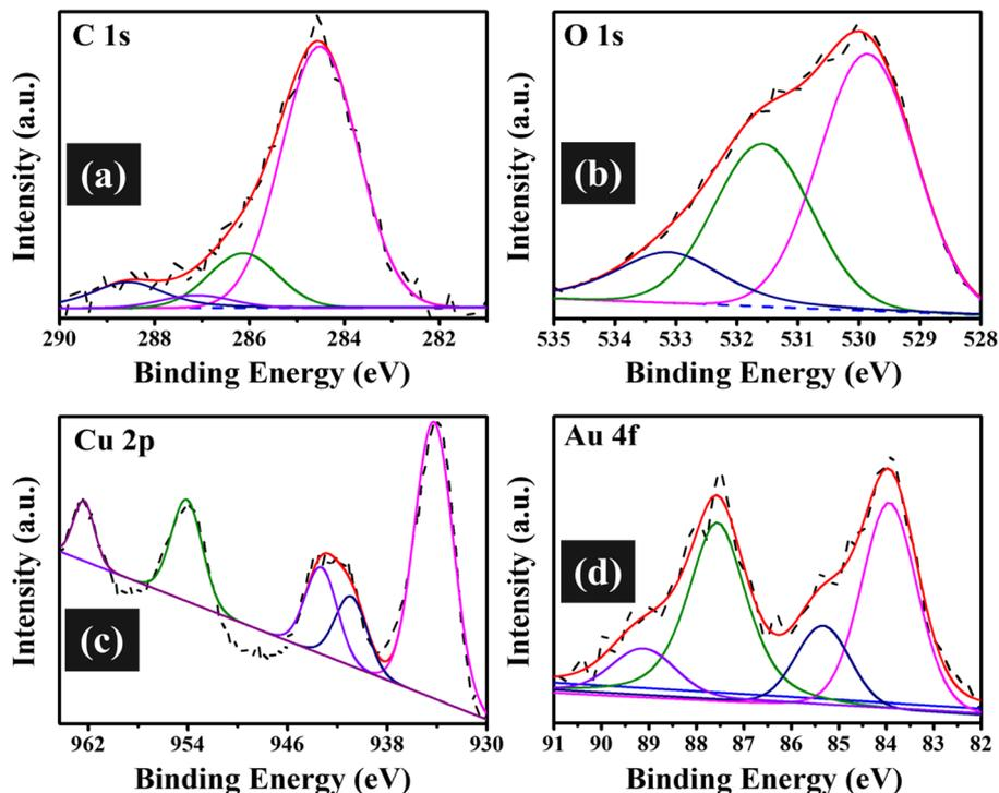
Fig. 2 XPS fine scan spectra of the Au@rGO/CuO nanocomposite: (a) C 1s, (b) O 1s, (c) Cu 2p, and (d) Au 4f.
