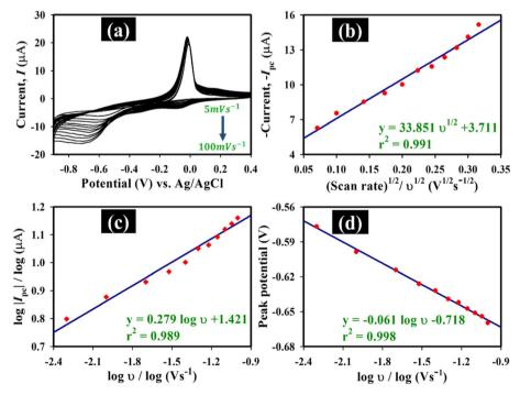
Fig. 8 (a) Voltammograms of Au@rGO/CuO/GCE at 30  $\mu$ m of MP in 0.1 M PBS (pH 7.0) obtained by varying the scan rate from 5 mV s<sup>-1</sup> to 100 mV<sup>-1</sup>. (b) Correlation between the square root of the scan rate ( $\nu$ ); and cathodic peak current ( $I_{pc}$ ); (c) correlation between log( $I_{pc}$ ) and log scan rate ( $\nu$ ); and (d) linear relationship between cathodic peak potential ( $E_p$ ) and log  $\nu$ .
