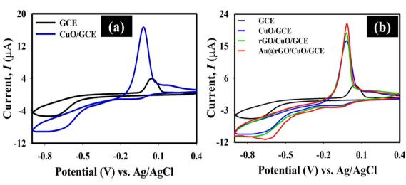
Fig. 6 Responses of CVs in the presence of 30  $\mu$ m MP in 0.1 M PBS: (a) bare GCE and CuO/GCE; (b) bare GCE, CuO/GCE, rGO/CuO/GCE, and Au@rGO/CuO/GCE at a scan rate of 50 mV s<sup>-1</sup>.
