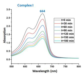
Fig. 6 Change in absorbance intensity of the MB dye at  $\lambda_{max}$  (664 nm) under visible light in the presence of compound I (5 mg). The MB concentration was 20 mg l<sup>-1</sup> with a pH of 6.
