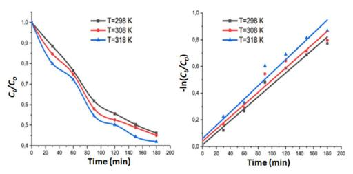
Fig. 10 Variation of  $C_t/C_o$  and  $-\ln(C_t/C_o)$  as a function of time at various temperatures. The lines represent the fitted data using the Pseudo-Second Order kinetic model.
