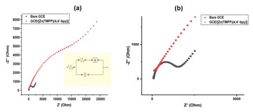
Fig. 12 (a) Nyquist plots were obtained for a 5 mM  $[Fe(CN)_6]^{3-/4}$  solution in 0.1 M of KCl of bare GCE and GCE/ $[Zn(TMPP)(4,4'-bpy)] \cdot CHCl_3$ . Measurements were conducted over a frequency range of 0.05 to 75 000 Hz. The inset illustrates the equivalent circuit model [(R(Q[RW]] used for data analysis.)] (b) Impedance graph with inset (0–5000 ohms).
