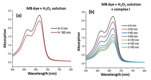
Fig. 11 Variation of the intensity of  $\lambda_{max}$  (664 nm) during the catalytic degradation of the MB dye in the presence of H<sub>2</sub>O<sub>2</sub> aqueous solution and the absence of complex I (a) and the presence of complex I (b).
