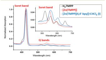
Fig. 1 UV-Vis spectra of  $H_2$ TMPP, [Zn(TMPP)] and [Zn(TMPP)(4,4′-bpy)]·CHCl $_3$  (I).
