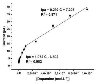
Fig. 16  $\,$  Plot of oxidation peak currents  $\it versus$  dopamine concentrations from 0 to  $\rm 10^{-4}~M.$
