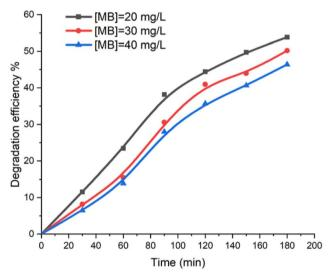
Fig. 9 Variation in color removal as a function of the initial dye concentration was examined under the following conditions: hydrogen peroxide concentration ( $C_0$ ) of 4 mL L<sup>-1</sup>, catalyst mass of 5 mg, and pH 6.
