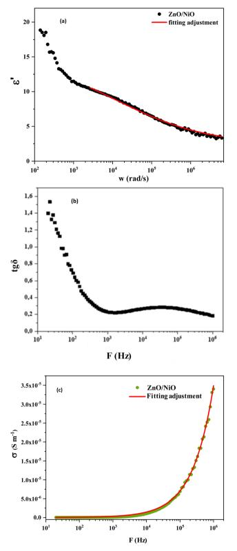
Fig. 7 (a) Variation of the dielectric constant as a function of frequency (b) variations of  $\tan\delta$  vs. frequency at room temperature (c) conductivity analysis: frequency-dependent behavior and relaxation processes.
