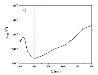
Fig. 5 (a) Variations of extinction coefficient and refractive index with wavelength (b) variation of optical conductivity ( $\sigma_{opt}$ ) vs. wavelength.
