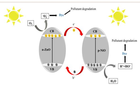
Fig. 10 The possible photocatalytic mechanism for ZnO/NiO photocatalyst.
