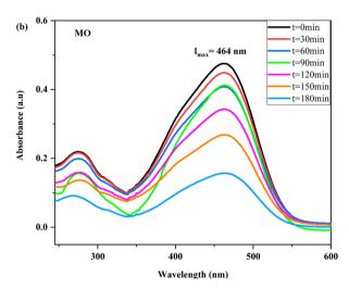
Fig. 8 UV-vis adsorption spectra as a function of degradation reaction time of (a) MB, and (b) MO aqueous solutions, catalyzed by the ZnO/ NiO powders under sunlight irradiation.
