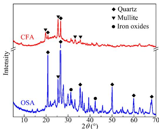
Fig. 1 XRD patterns of OSA and CFA.
