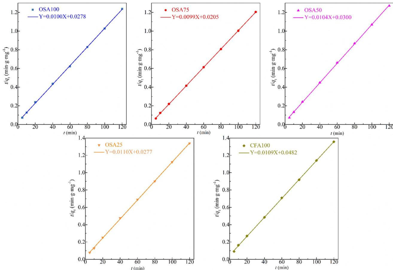
Fig. 7 Pseudo-second-order kinetic model for  $\text{Cd}^{2+}$  adsorption onto zeolites.
