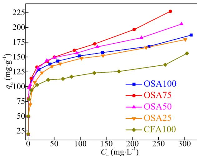
Fig. 8 Influence of initial  $\text{Cd}^{2+}$  concentration on adsorption behavior of zeolites ( $m = 1 \text{ g L}^{-1}$ ,  $\text{pH} = 7$ ,  $t = 60 \text{ min}$ ,  $T = 30 \text{ }^\circ\text{C}$ ).
