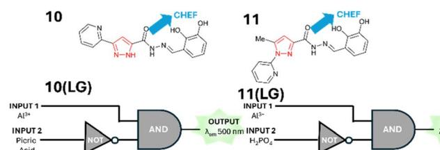
Fig. 13 Pyridine-based pyrazole 10 and 11 and their application as logic gates 10(LG) and 11(LG).<sup>36,37</sup>
