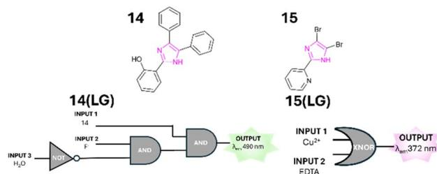
Fig. 16 Diphenyl-imidazole **14** and pyridine-imidazole **15** and their corresponding logic gates **14(LG)** and **15(LG)**.<sup>41,42</sup>
