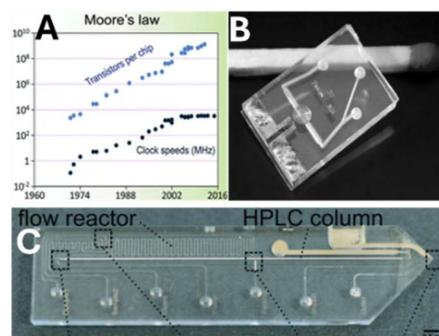
Fig. 1 Approaching the end of Moore's law (panel A),<sup>7b</sup> a lab-on-chip NMR (panel B)<sup>8c</sup> and HPLC (panel C).<sup>9</sup> Images reproduced from ref. 7b, 8c and 9 with permission from RSC, copyright 2019, 2005 and 2017 respectively.
