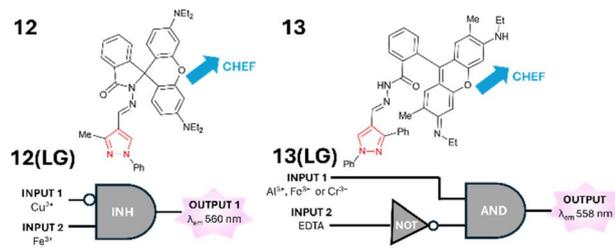
Fig. 14 Rhodamine-pyrazole **12** and **13** and their application as logic gates **12(LG)** and **13(LG)**.<sup>38,39</sup>
