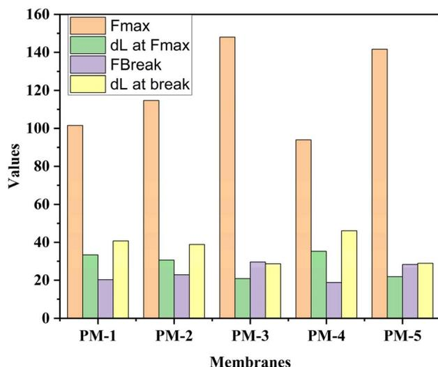
Fig. 10 Comparison of the mechanical properties of the membranes (PM-1 to PM-5).
