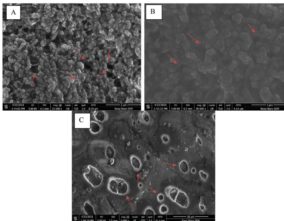
Fig. 7 Surface analysis of the PP membrane at 25 000 $\times$  magnification (A), surface analysis of the PP membrane at 500 00 $\times$  (B) with a working distance (WD) of 4.2 mm, and surface analysis of the PP membrane at 500 00 $\times$  (C) with a working distance (WD) of 3.5 mm.
