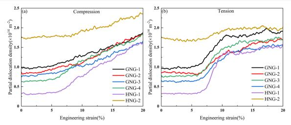
Fig. 15 Evolution of the partial dislocation density in HEA under different loads. (a) Compression. (b) Tension.
