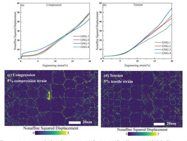
Fig. 6 NSD curves and cloud maps of G-HEA. (a) Compressive load. (b) Tensile load. (c) The NSD cloud map of GNG-3 at 5% compressive strain. (d) The NSD cloud map of GNG-3 at 5% tensile strain.
