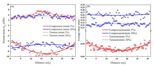
Distribution of the average normal stress and shear strain in GNG-3. (a) Normal stress  $\sigma_{VV}$ . (b) Average shear strain
