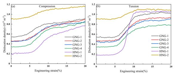
Evolution curves of the dislocation densities in GNG-3 under different loads. (a) Compression. (b) Tension.
