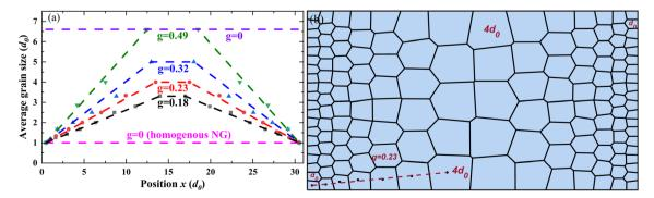
Fig. 1 (a) Variation in the average grain size of polycrystalline HEA along the x-axis, showing smaller average grain sizes in the regions on both sides and larger grain sizes in the central region. Four linear gradients and two uniform HEA atomic models were constructed. (b) Microstructural morphology of the model with a gradient of q = 0.23, where  $d_0$  represents the minimum grain size.
