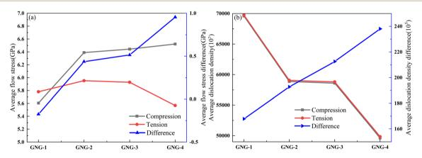
Fig. 14 Average flow stresses and average dislocation densities of GNG HEA. (a) Average flow stress. (b) Average dislocation density.
