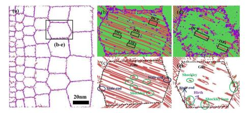
Fig. 10 Microstructures and dislocations of the GNG-3 under different loads. (a) The left half of the atomic model before loading. (b) and (c) The enlarged view at  $\varepsilon=10\%$  under compression. (d) and (e) The enlarged view at  $\varepsilon=10\%$  under tension. The four images on the right are enlarged views of the same grain selected by the rectangular box in (a). Among them, green, red, and purple represent FCC, HCP, and GBs respectively, and the back dashed line is also GBs.
