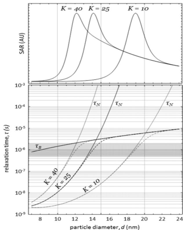
Fig. 10 Effect of anisotropy on relaxation time and SAR. Copyright 2014, Elsevier.<sup>194,250</sup>
