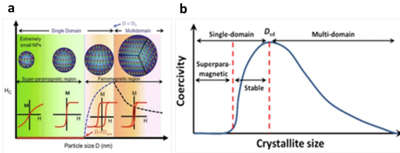
Fig. 3 (a and b) Dependence of magnetization on size of IONPs. Copyright 2005 & 2018, Elsevier.<sup>58,59</sup>
