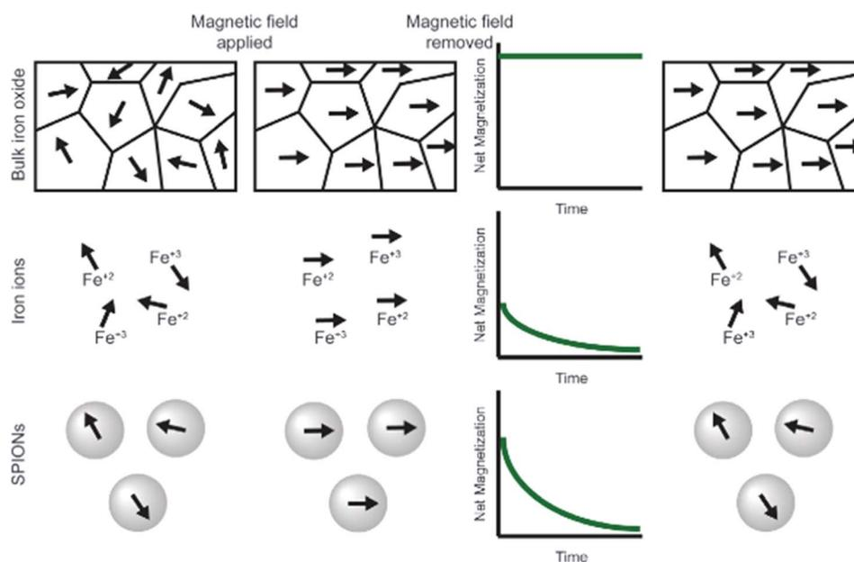
Fig. 2 Effect of external magnetic field on the net magnetization of bulk magnetite, iron ions, and SPIONs. Copyright 2011, Elsevier.<sup>50</sup>
