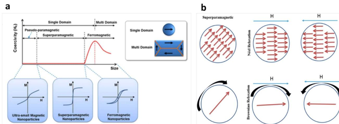
Fig. 9 Hysteresis loop (a) Brownian relaxation USM NPs, superparamagnetic, and ferromagnetic nanoparticles (b) of superparamagnetic NPs. Copyright 2017, Springer Nature.<sup>243,244</sup>
