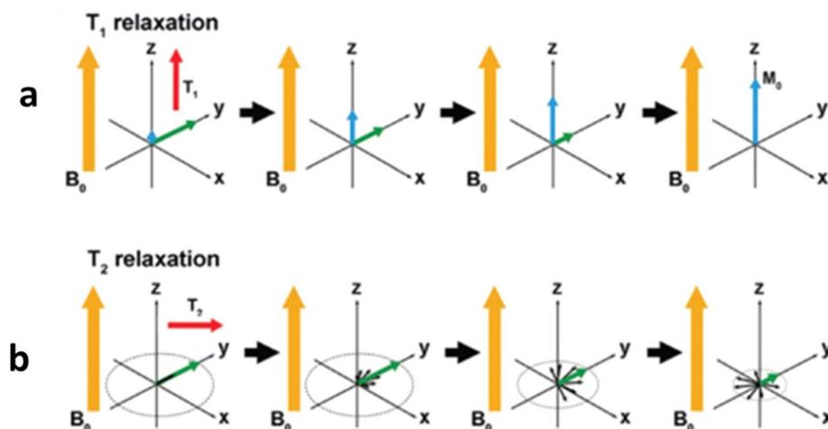
Fig. 5 Mechanism of  $T_1$  relaxation and  $T_2$  relaxation<sup>67</sup>
