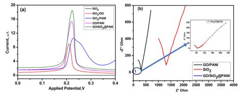
Fig. 3 (a) Shows the differential pulse voltametric sensing of dopamine of  $12 \mu M$  concentration using SiO<sub>2</sub>, SiO<sub>2</sub>/GO, SiO<sub>2</sub>/PANI, GO/PANI and GO/SiO<sub>2</sub>@PANI modified GCE (PBS buffer) (b) EIS analysis of 5 mM of K<sub>4</sub>[Fe (CN)<sub>6</sub>] with 0.1 M KCl using GO/PANI, SiO<sub>2</sub> and GO/SiO<sub>2</sub>@PANI to determine the charge transfer resistance.
