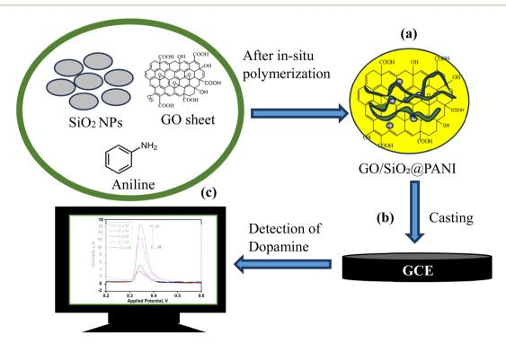
Fig. 1 (a) Synthesis of GO/SiO<sub>2</sub>@PANI, (b) fabrication of GO/SiO<sub>2</sub>@PANI on GCE electrode surface, and (c) detection of dopamine using GO/ SiO<sub>2</sub>@PANI as an electrochemical sensor.
