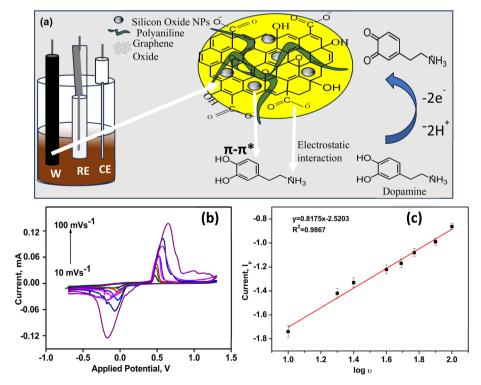
Fig. 4 (a) Scheme demonstrate the mechanism for detection of dopamine using  $GO/SiO_2@PANI$  as an electrochemical sensing probe that were fabricated on the GCE; (b) CVs of 12  $\mu$ M/0.1 M PBS buffer (pH = 7.4) at  $GO/SiO_2@PANI$  at different scan rate from 10–100 mV s<sup>-1</sup> (c) showing the result of variation of log of oxidation peak current for 12  $\mu$ M concentration of dopamine *versus* log of scan rate.
