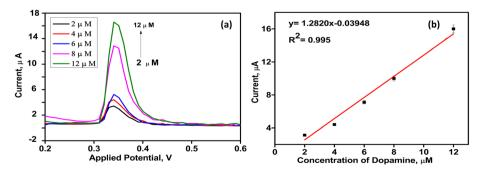
Fig. 5 (a) DPV peaks for different concentrations of dopamine from 2 to 12  $\mu$ M with PBS buffer (pH 7.4) and (b) standard calibration curve for respective dopamine concentrations.
