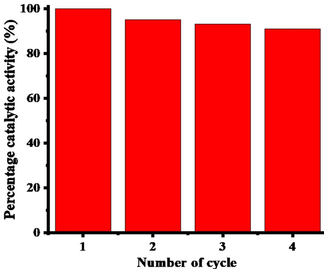
Fig. 9 Catalytic activity during recycling [conditions: [4NBA] = 0.049 mM, Ag-AN-P(NM) = 1.48 mg mL<sup>-1</sup>, and [BH<sub>4</sub><sup>-</sup>] = 3.55 mM].
