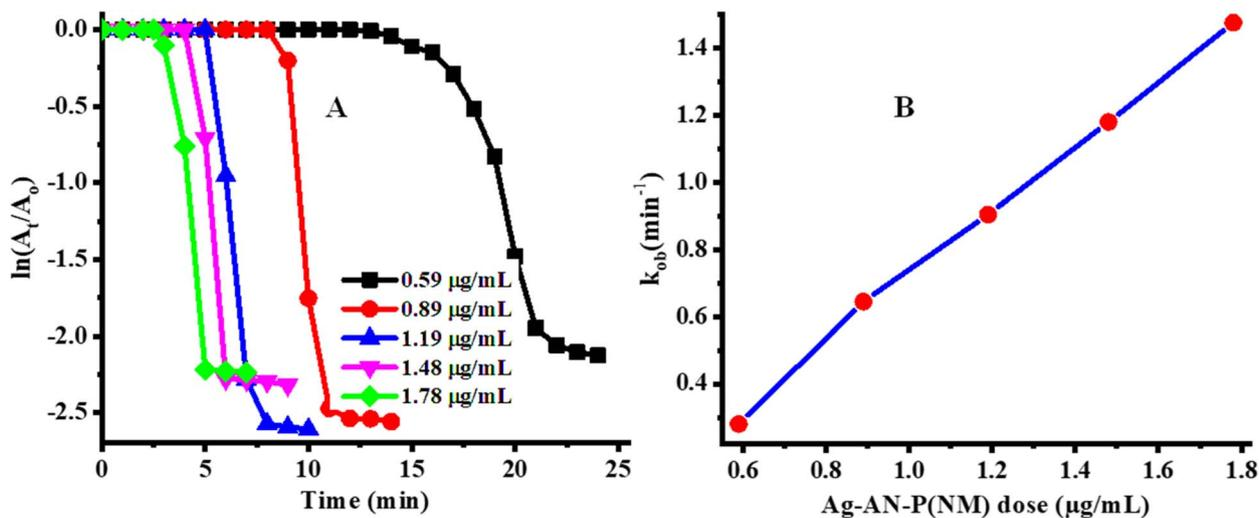
Fig. 6 Catalytic reduction of 4NBA: (A) effect of the amount of the catalyst [conditions: Ag-AN-P(NM) = 0.59–1.78 mg mL<sup>-1</sup>, [4NBA] = 0.049 mM, and [NaBH<sub>4</sub>] = 3.55 mM] (B) graph between  $k_{\text{ob}}$  and catalytic dose.
