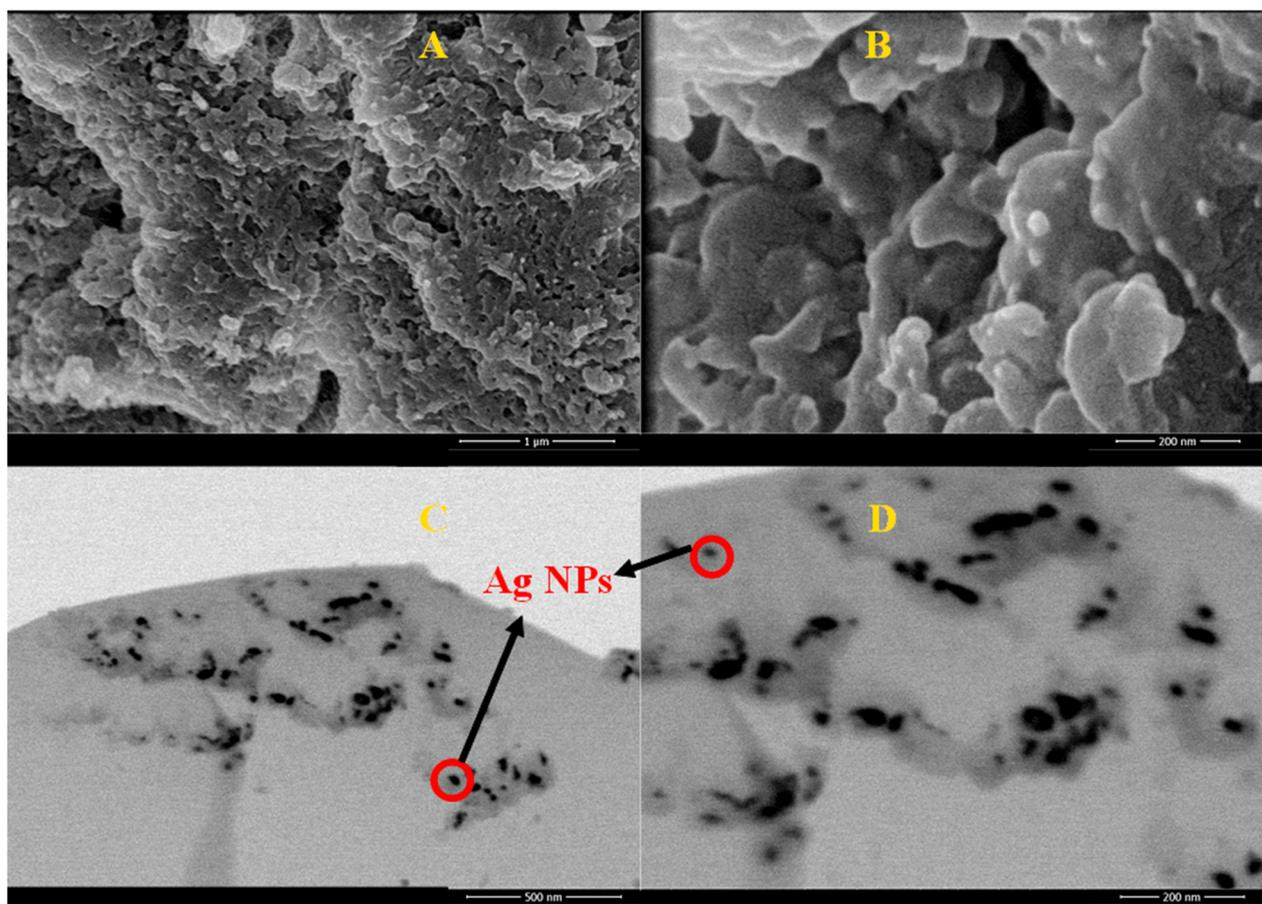
Fig. 4 (A and B) SEM results of AN-P(NM) and (C and D) TEM images of Ag-AN-P(NM).
