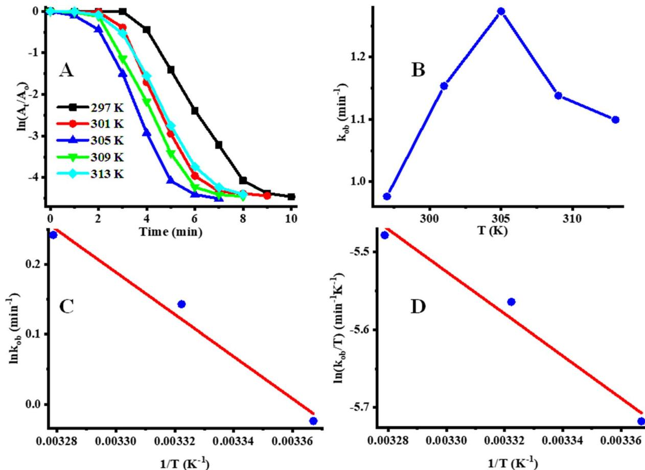
Fig. 7 Catalytic reduction of 4NBA under different temperatures (297–313 K) illustrated as follows: (A) time vs.  $\ln(A_t/A_0)$  under different temperatures [conditions: 4NBA concentration = 0.049 mM,  $[\text{NaBH}_4] = 3.55$  mM, and  $\text{Ag-AN-P(NM)} = 1.48$  mg  $\text{mL}^{-1}$ ], (B)  $k_{\text{ob}}$  vs. temperature, (C) Arrhenius, and (D) Eyring plot.
