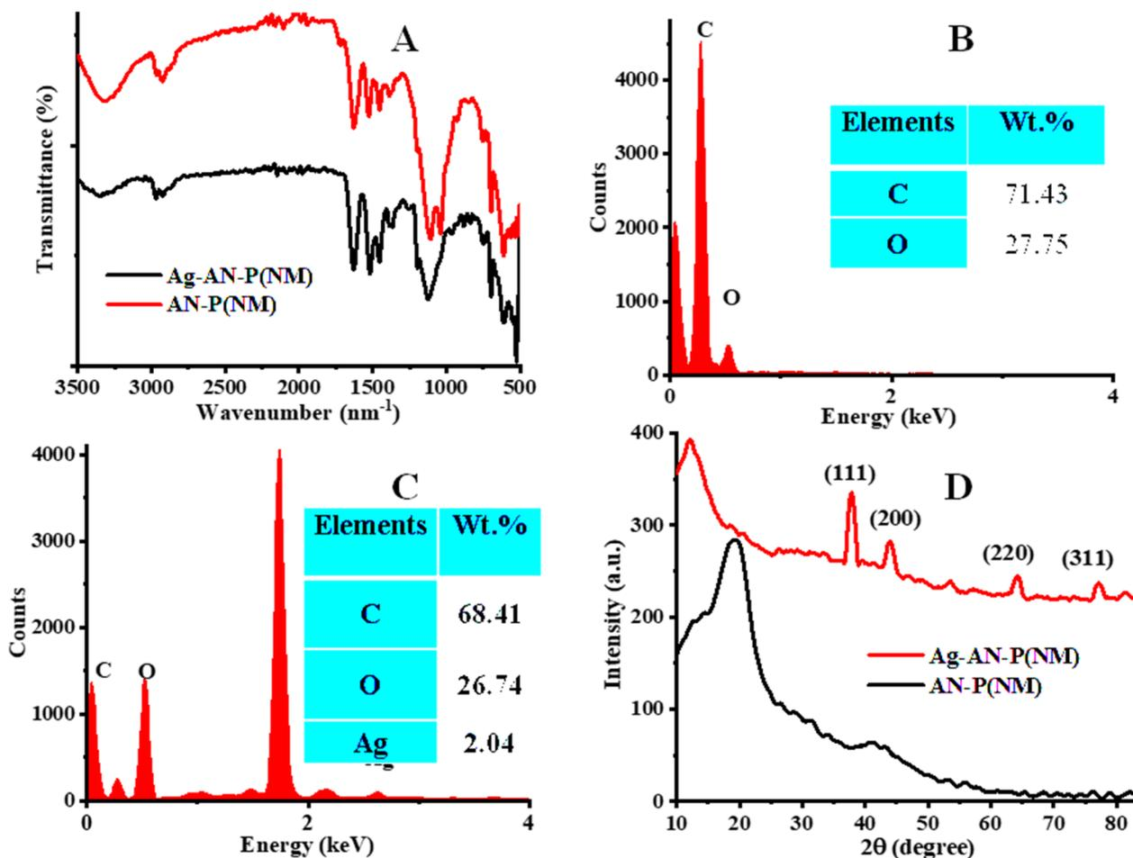
Fig. 2 (A) FTIR spectra of AN-P(NM) and Ag-AN-P(NM), (B and C) EDX results of AN-P(NM) and Ag-AN-P(NM), respectively, and (D) XRD spectra of AN-P(NM) and Ag-AN-P(NM).
