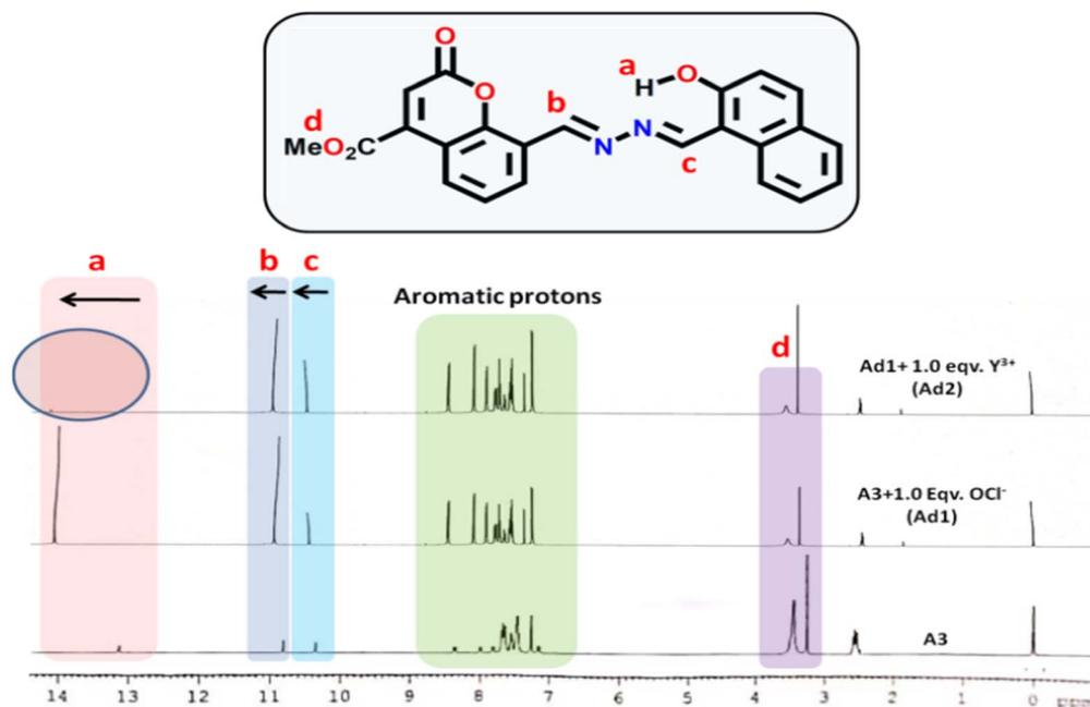
Fig. 6 Changes in the <sup>1</sup>H-NMR spectra of **A3** upon addition of  $\text{OCl}^-$  and  $\text{Y}^{3+}$  in a cascade manner (solvent,  $\text{CDCl}_3$ ).
