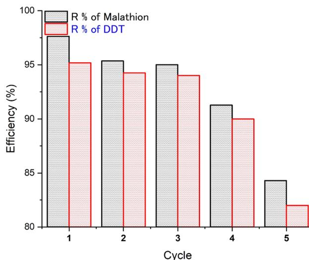
Fig. 9 Different reusability cycles of the N-Bent-NAl<sub>2</sub>O<sub>3</sub>-NZnO nanocomposite for malathion and DDT adsorption at the contact time of 80 min, initial pH value of 3.0, initial concentration of 40.0 mg L<sup>-1</sup> and shaking speed of 240 rpm.
