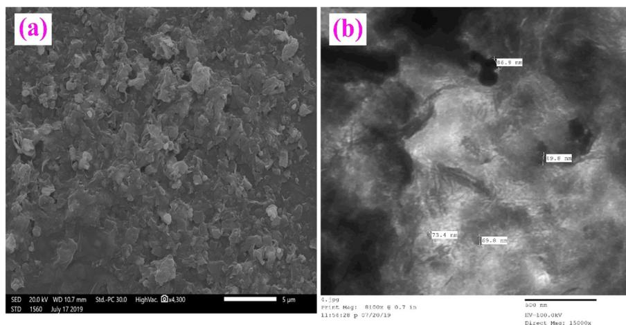
Fig. 4 (a) SEM and (b) HR-TEM images of the N-Bent-NAL<sub>2</sub>O<sub>3</sub>-NZnO nanocomposite.
