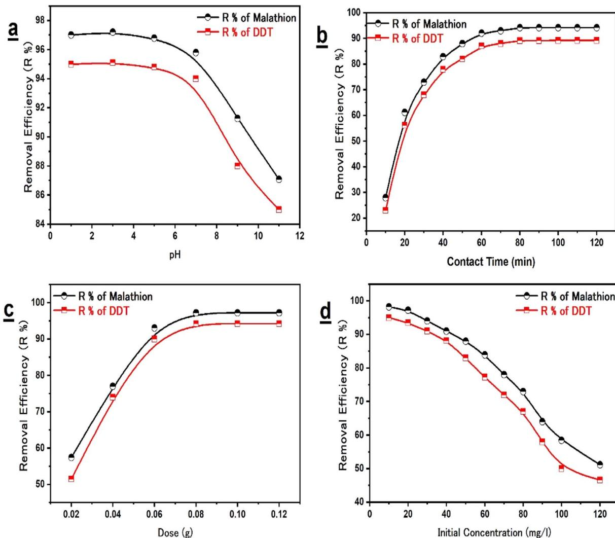
Fig. 6 Effect of (a) initial solution pH, (b) contact time, (c) nanocomposite dose, and (d) initial organic pollutant concentration on the removal efficiency ( $R\%$ ) of malathion and DDT adsorption by N-Bent-NaAl<sub>2</sub>O<sub>3</sub>-NZnO. (Sample volume = 10.0 mL; nanocomposite dose = 40.0 ± 1.0 mg; malathion & DDT initial concentrations = 40.0 mg L; initial pH value = 3.0; shaking time = 80 min; temperature = 25.0 ± 1.0 °C; shaking speed = 240 rpm).
