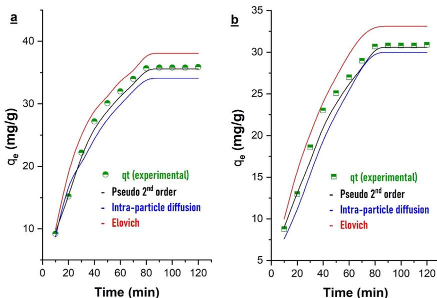
**Fig. 7** Kinetics models (Pseudo second order, Intra-particle diffusion and Elovich kinetic model) for (a) malathion and (b) DDT adsorption onto the N-Bent-NAL<sub>2</sub>O<sub>3</sub>-NZnO nanocomposite at 25 °C.
