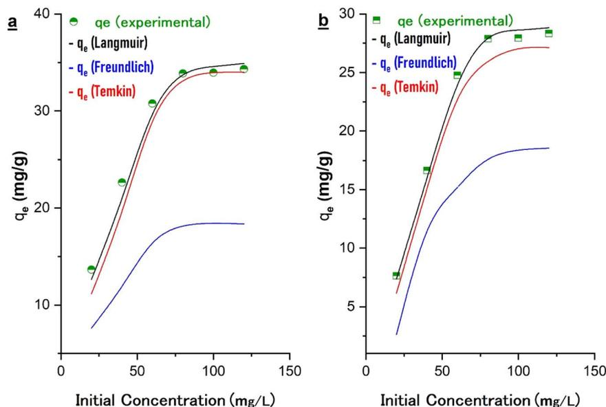
Fig. 8 Langmuir, Freundlich and Temkin isothermal models for (a) malathion and (b) DDT adsorption onto the N-Bent-NAl<sub>2</sub>O<sub>3</sub>-NZnO nanocomposite at 25 °C.
