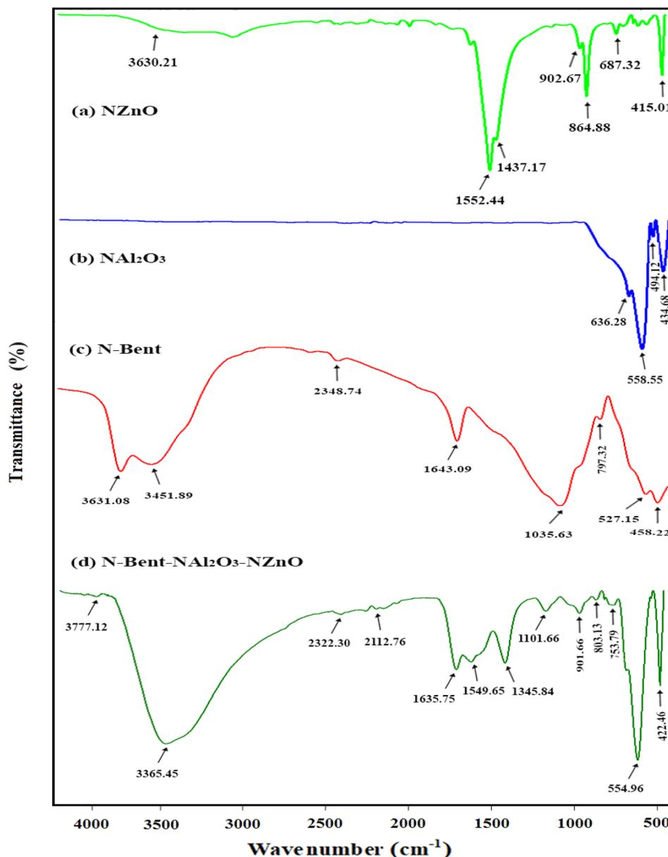
Fig. 1 FT-IR spectra of (a) NZnO, (b) NAl<sub>2</sub>O<sub>3</sub>, (c) N-Bent, and (d) the N-Bent-NAl<sub>2</sub>O<sub>3</sub>-NZnO nanocomposite.
