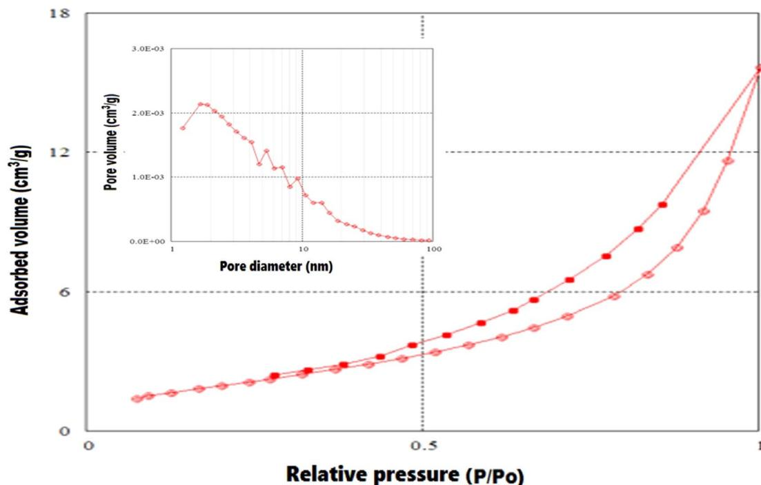
Fig. 5 Nitrogen adsorption–desorption isotherm of the N-Bent-NAl<sub>2</sub>O<sub>3</sub>-NZnO nanocomposite. The inset shows the pore size.
