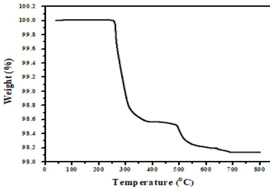
Fig. 3 TGA thermogram of the N-Bent-NAL<sub>2</sub>O<sub>3</sub>-NZnO nanocomposite.
