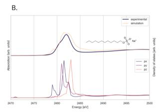
Fig. 10 (A) Experimental absorption data and spectra of IPTG simulated with FDMNES (left axis), correlated with the density of states (right axis), showing the occupancy of different molecular orbitals present in the molecule. (B) Experimental and simulated spectra of SDS, and electronic transitions in the orbitals responsible for the features in the spectrum.
