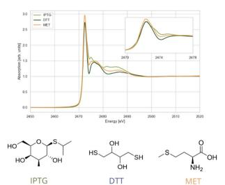
Fig. 3 Sulphur K-edge XANES spectra of compounds with sulphur environment R-S-R; IPTG (isopropyl- $\beta$ -D-thiogalactopyranoside), DTT (dithiothreitol), MET (methionine). The inset displays the white lines at a larger scale.
