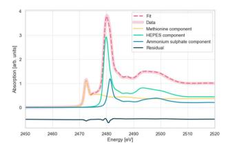
Fig. 9 Sulphur K-edge XANES spectra of reference compounds compared to the spectrum of a mixture of these substances (red) and the result of linear combination fitting (dotted red).
