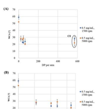
Fig. 4 WCA as a function of DP per arm of obtained polymers at a concentration of  $0.5 \text{ mg mL}^{-1}$  (A), a subset of the top graph showing only star-shaped polymers (B).
