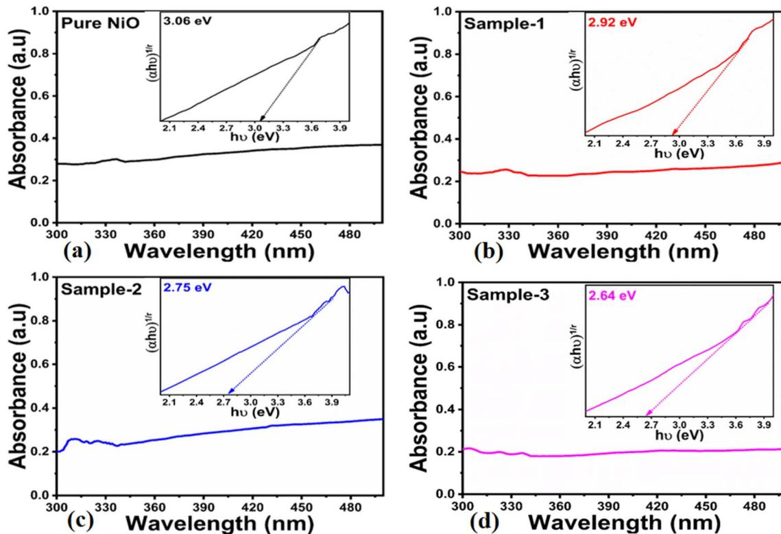
Fig. 2 UV-visible absorption spectra of (a) pure NiO and (b–d) NiO/MgO–SiO<sub>2</sub> composites (sample 1 and sample 2).
