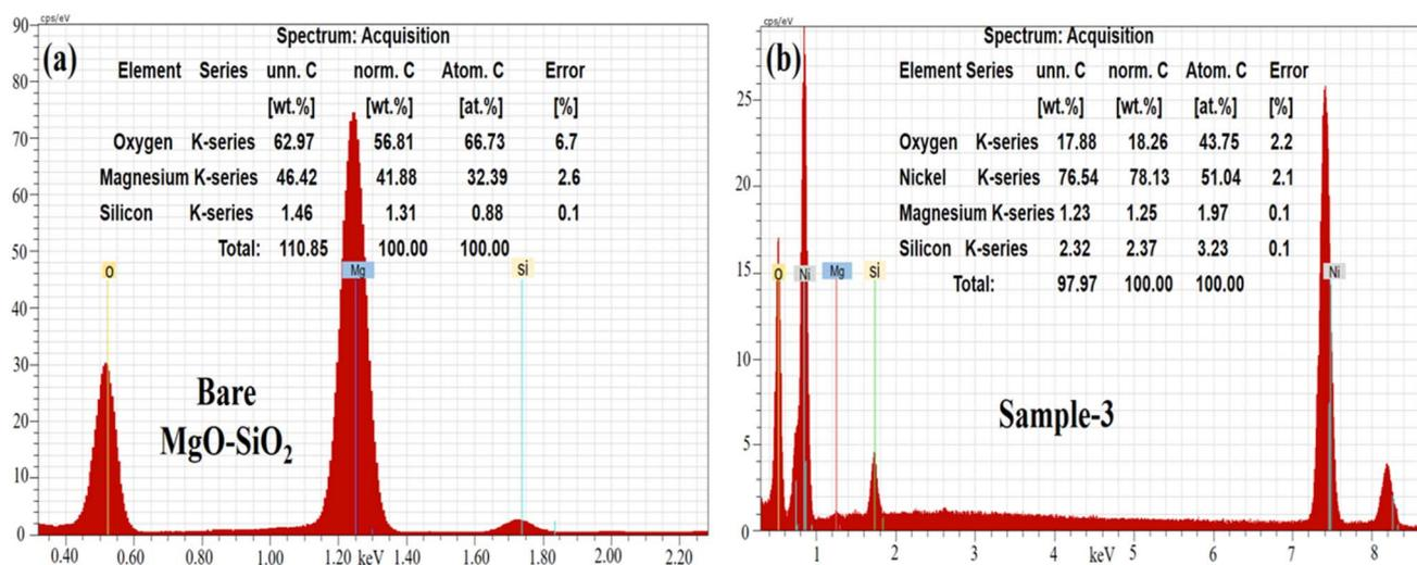
Fig. 4 EDX spectra of the (a) bare MgO–SiO<sub>2</sub> composite and (b) NiO/MgO–SiO<sub>2</sub> composites (sample 3).
