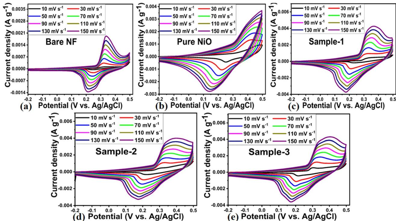
Fig. 7 CV curves of (a) bare nickel foam, (b) pure NiO, (c) MgO–SiO<sub>2</sub> composites (sample 1), and (d and e) NiO/MgO–SiO<sub>2</sub> composites (sample 2 and sample 3) using different scan rates in electrolytic solution of 3 M KOH for the illustration of capacitance performance of each electrode material.
