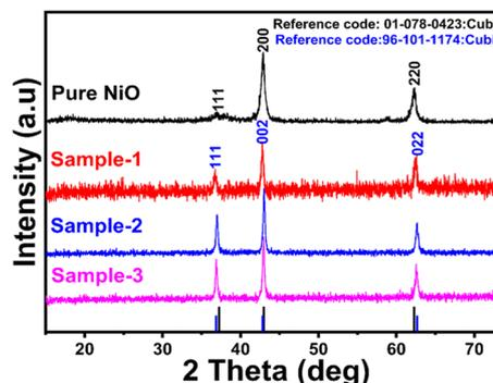
Fig. 1 Diffraction patterns measured by XRD for pure NiO and NiO/MgO–SiO<sub>2</sub> composites (sample 1 and sample 2).
