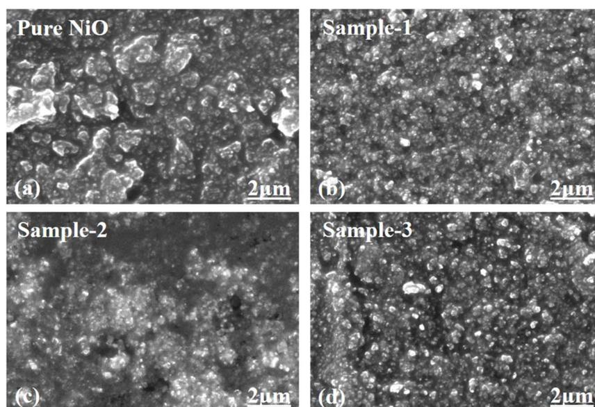
Fig. 3 Distinctive SEM images of (a) pure NiO, (b) MgO–SiO<sub>2</sub> composites (sample 1) and (c and d) NiO/MgO–SiO<sub>2</sub> composites (sample 2 and sample 3).
