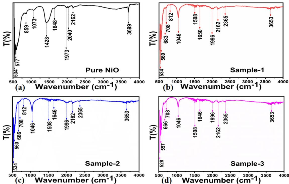
Fig. 5 FTIR spectra of (a) pure NiO, (b) MgO-SiO<sub>2</sub> composites (sample 1), and (c and d) NiO/MgO-SiO<sub>2</sub> composites (sample 2 and sample 3).
