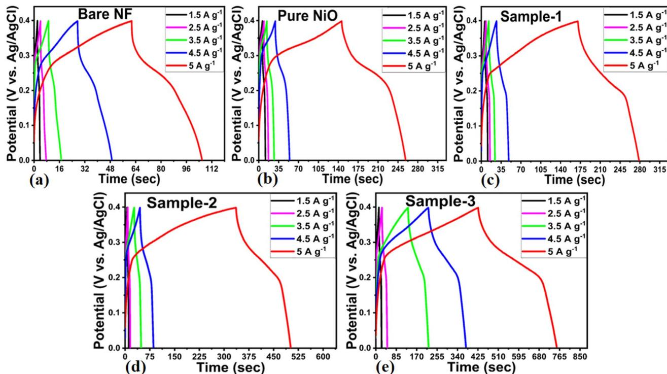
Fig. 8 Galvanic charge–discharge cycles of (a) bare nickel foam, (b) pure NiO, (c) MgO–SiO<sub>2</sub> composites (sample 1), (d and e) NiO/MgO–SiO<sub>2</sub> composites (sample 2 and sample 3) using current densities from 1.5 to 5 A g<sup>-1</sup> in an electrolytic solution of 3 M KOH for the illustration of capacitance performance of each electrode material.
