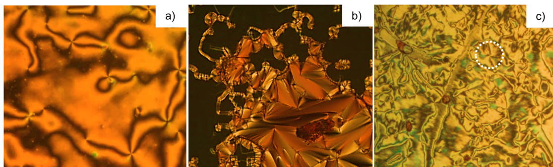
Fig. 7 POM textures observed for: (a) HHH8 in the nematic phase at 128 °C, (b) HHH14 in the SmA phase at 120 °C and (c) HHH12 in the synclinic SmC phase at 105 °C.
