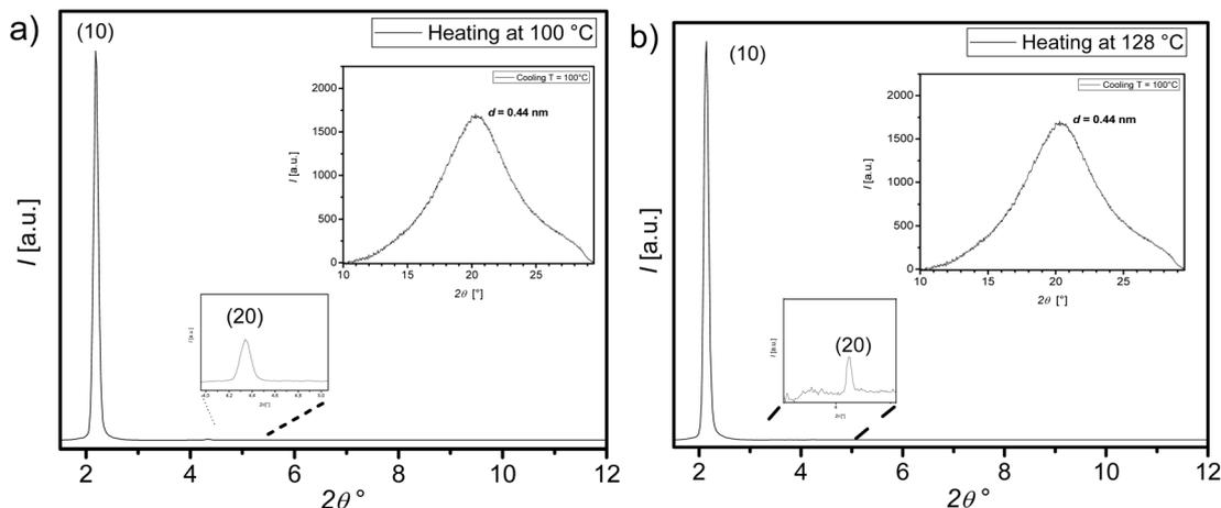
Fig. 10 Plot of the integrated scattered intensity as a function of  $2\theta$  in the small-angle region (SAXS) for HHH14: (a) the SmC phase at  $T = 100$  °C and (b) the SmA phase at  $T = 128$  °C. The insets in (a) and (b) show the WAXS region in both phases.
