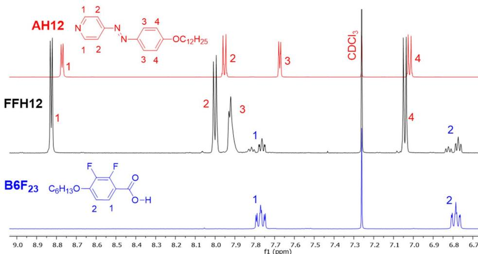
Fig. 4  $^1\text{H}$  NMR spectra (500 MHz,  $\text{CDCl}_3$ ) of the supramolecule **FFH12** (black) and its complementary components the azopyridine derivative **AH12** (red) and the benzoic acid derivative **B6F<sub>23</sub>** (blue) in the aromatic region (for the whole range see Fig. S20 $\dagger$  in the ESI).
