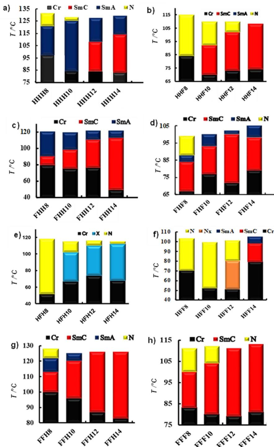
Fig. 6 Schematic illustration of combined DSC and POM data on cooling at a rate of  $10 \text{ K min}^{-1}$  for the synthesized HBLCs. N = nematic phase, SmA = smectic A, SmC = smectic C, X = unknown LC phase; Nx = nematic x phase.
