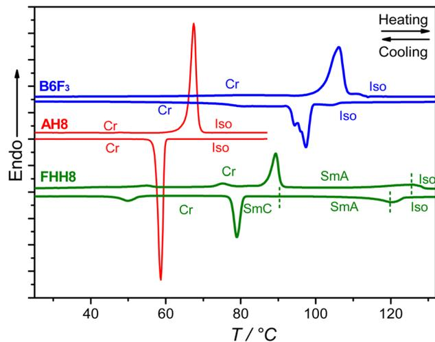
Fig. 5 DSC Heating and cooling cycles of the HBL C FHH8 (green curves) and its individual components, the proton donor B6F<sub>3</sub> (blue curves) and the proton acceptor AH8 (red curves) at a scanning rate of 10 K min<sup>-1</sup>.
