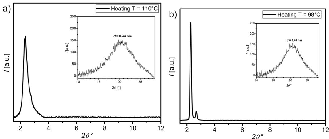
Fig. 11 Plot of the integrated scattered intensity as a function of  $2\theta$  in the small-angle region (SAXS) for HFH10 on cooling: (a) the N phase at  $T = 110^\circ\text{C}$ , (b) the X phase at  $T = 98^\circ\text{C}$ . The insets in (a) and (b) show the WAXS region in both phases.
