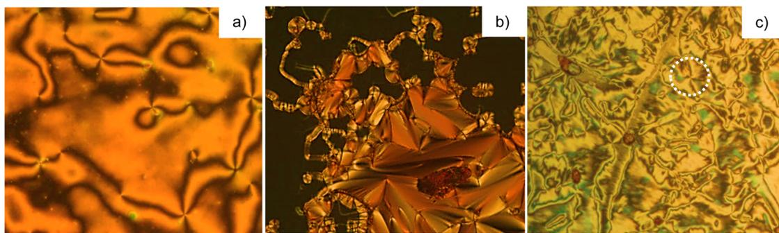
Fig. 7 POM textures observed for: (a) HHH8 in the nematic phase at 128 °C, (b) HHH14 in the SmA phase at 120 °C and (c) HHH12 in the synclinc SmC phase at 105 °C.
