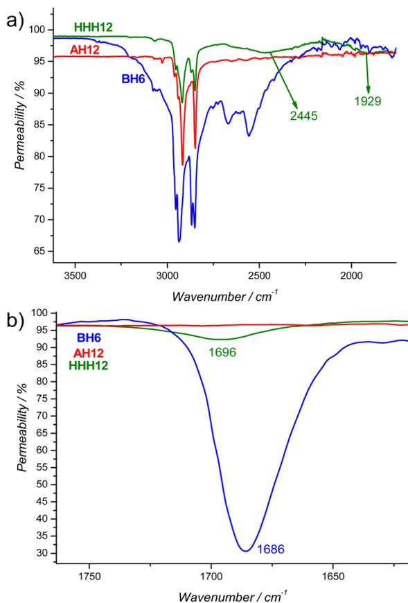
Fig. 2 FTIR spectra of the supramolecule **HHH12** (green) and its complementary components **B6H** (blue), **AH12** (red) in the crystalline state at room temperature enlarged area (a) between 1750  $\text{cm}^{-1}$  and 3600  $\text{cm}^{-1}$  and (b) between 1620  $\text{cm}^{-1}$  and 1760  $\text{cm}^{-1}$ .
