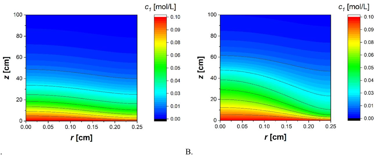
Fig. 7 Contour diagrams for the glucose concentration profiles calculated with (A) Wilke–Chang correlation and (B) Taylor method.
