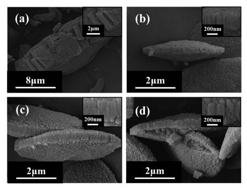
Fig. 2 SEM images of H-type samples with different ratios of OH<sup>-</sup>/SiO<sub>2</sub> ((a) 0.25\*; (b) 0.15; (c) 0.2; (d) 0.25) (\*without seeds).
