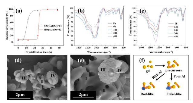
Fig. 12 (a) Crystallization curves of samples ( $SiO_2/Al_2O_3 = 14$  and 42); (b and c) FT-IR spectra of samples ( $SiO_2/Al_2O_3 = 14$  and 42); (d and e) SEM images of samples ( $SiO_2/Al_2O_3 = 14$  and 42); (f) comparison of growth processes.
