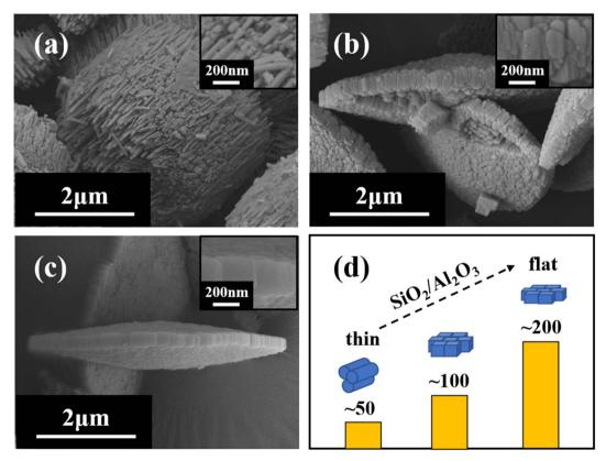
Fig. 4 SEM images of H-type samples with different ratios of SiO<sub>2</sub>/Al<sub>2</sub>O<sub>3</sub> ((a) 14; (b) 21; (c) 28) and process of layer width transformation (d).
