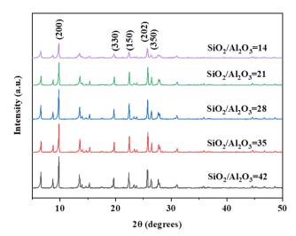
Fig. 5 XRD patterns of H-type samples with different ratios of SiO<sub>2</sub>/ Al<sub>2</sub>O<sub>3</sub> (170 °C).
