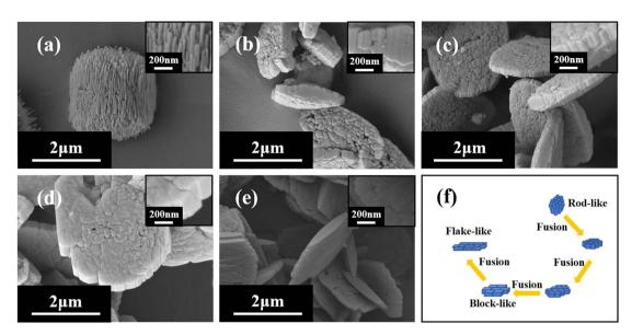
Fig. 6 SEM images of H-MOR with different ratios of SiO<sub>2</sub>/Al<sub>2</sub>O<sub>3</sub> ((a) 14; (b) 21; (c) 28; (d) 35; (e) 42) and transformation process (f).
