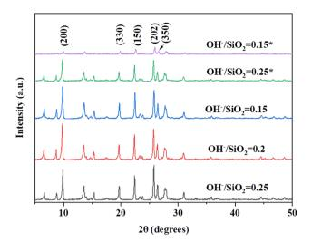
Fig. 1  $\,$  XRD patterns of H-type samples with different ratios of OH $^-/$  SiO $_2$  (\*without seeds).
