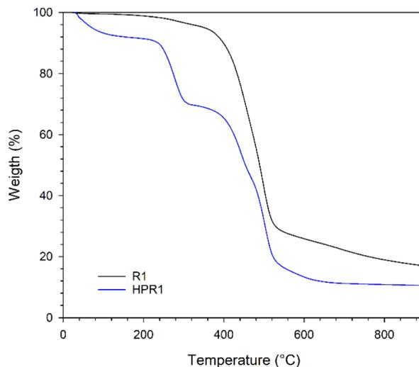
Fig. 4 TGA curves of the R1 resin and HPR1 resin synthesized in a single step.
