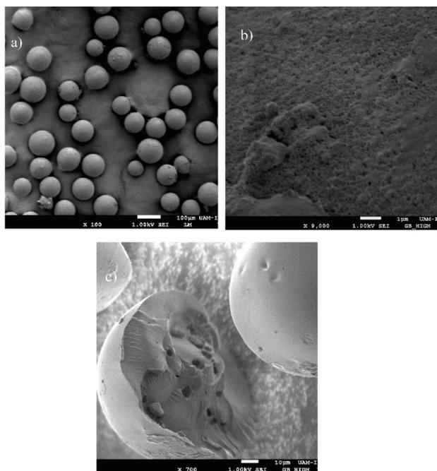
Fig. 1 Scanning Electron Microscopy (SEM) Images of synthesized resins. (a) Spherical particles obtained through suspension polymerization of the R1 resin. (b) The surface of a single particles of the HPR1 resin (c) morphology of cleaved particles after the post-crosslinked of the HPR1 resin.
