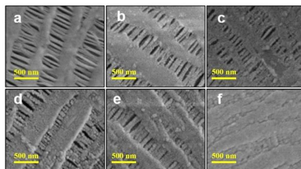
Fig. 5 SEM images showing immaculate (a) and porous polypropylene hollow fibre membrane with the deposition of Al<sub>2</sub>O<sub>3</sub> at (b) 50, (c) 100, (d) 200, (e) 300, and (f) 400 cycles (reprinted with permission from ref. 48 copyright 2017, The Chemical Industry and Engineering Society of China, and Chemical Industry Press).
