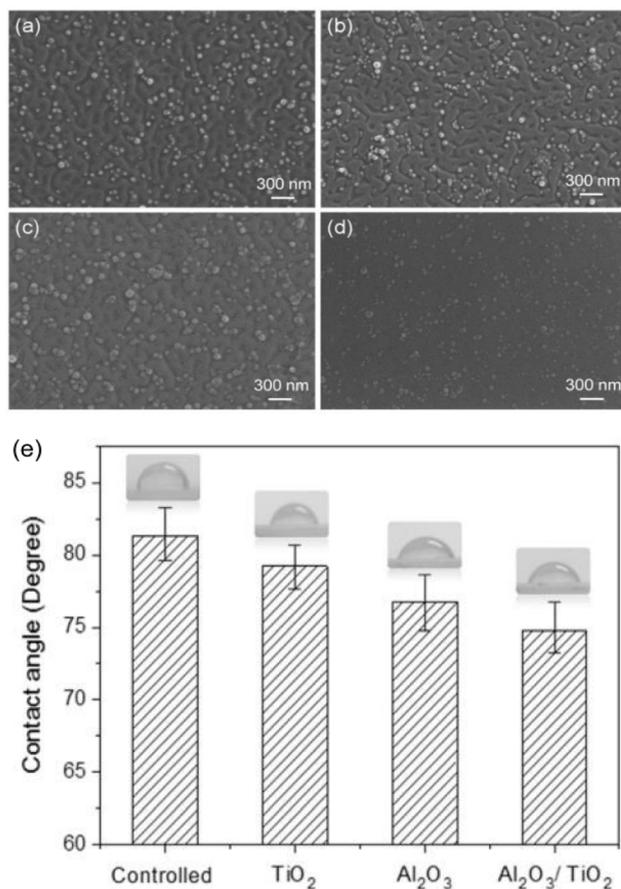
Fig. 7 SEM images of (a) PET without coating and PET surface with coatings of (b) TiO<sub>2</sub>, (c) Al<sub>2</sub>O<sub>3</sub> after 100 cycles of ALD, and (d) Al<sub>2</sub>O<sub>3</sub>/TiO<sub>2</sub> multilayer with 100 cycles of ALD for each layer. (e) Contact angles for the oxide-coated PET and uncoated PET (reprinted with permission from ref. 119 Copyright 2017, Elsevier B.V.).
