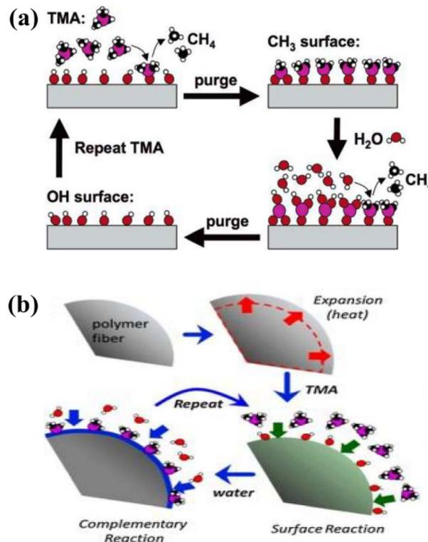
Fig. 8 (a) Diagram of an ALD cycle, self-limited ALD, showing layer-by-layer controllable construction of an Al<sub>2</sub>O<sub>3</sub> layer from TMA and H<sub>2</sub>O precursors (reprinted with permission from ref. 133 copyright 2007, the American Chemical Society). (b) Cotton fiber surface with abundant -OH groups exposed to ALD (reprinted with permission from ref. 12 copyright 2013, Elsevier B.V.).
