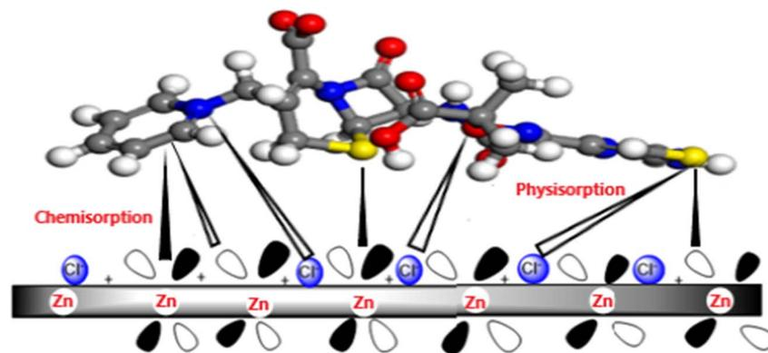
Fig. 11 Proposed mechanism of the Ceftazidime drug as a corrosion inhibitor for zinc metal.
