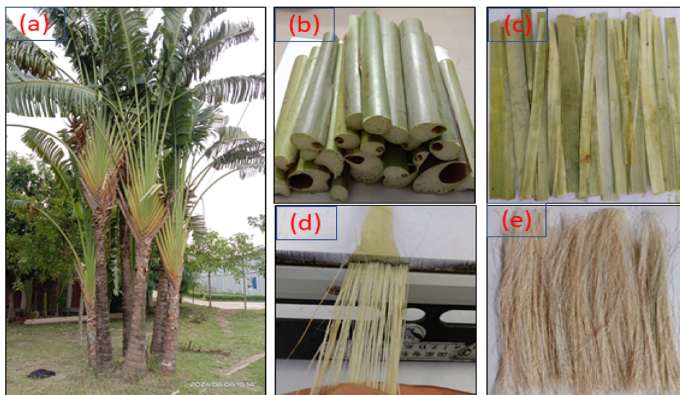
Fig. 1 RMF extraction process: (a) R. madagascariensis plant, (b) collected leaf stalks, (c) removed spongy parts of leaf stalks, (d) mechanical retting, and (e) extracted fibers.
