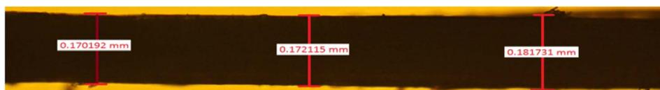
Fig. 2 Optical microscope image of the RMF.
