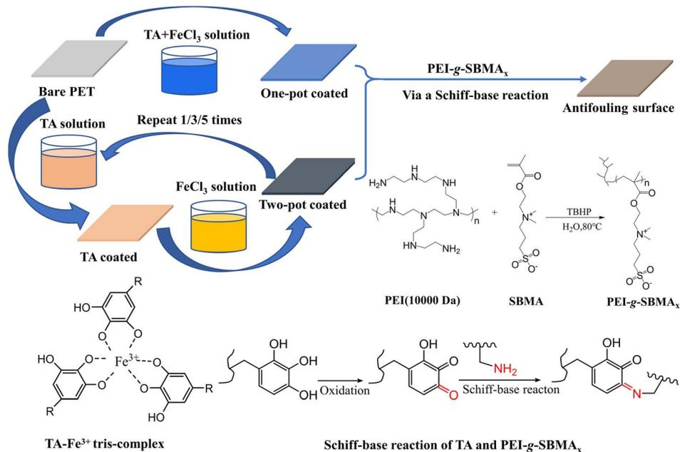
Scheme 1 Preparation process of antifouling PEI-g-SBMA<sub>x</sub>/TA-Fe<sup>3+</sup>/PET composite.
