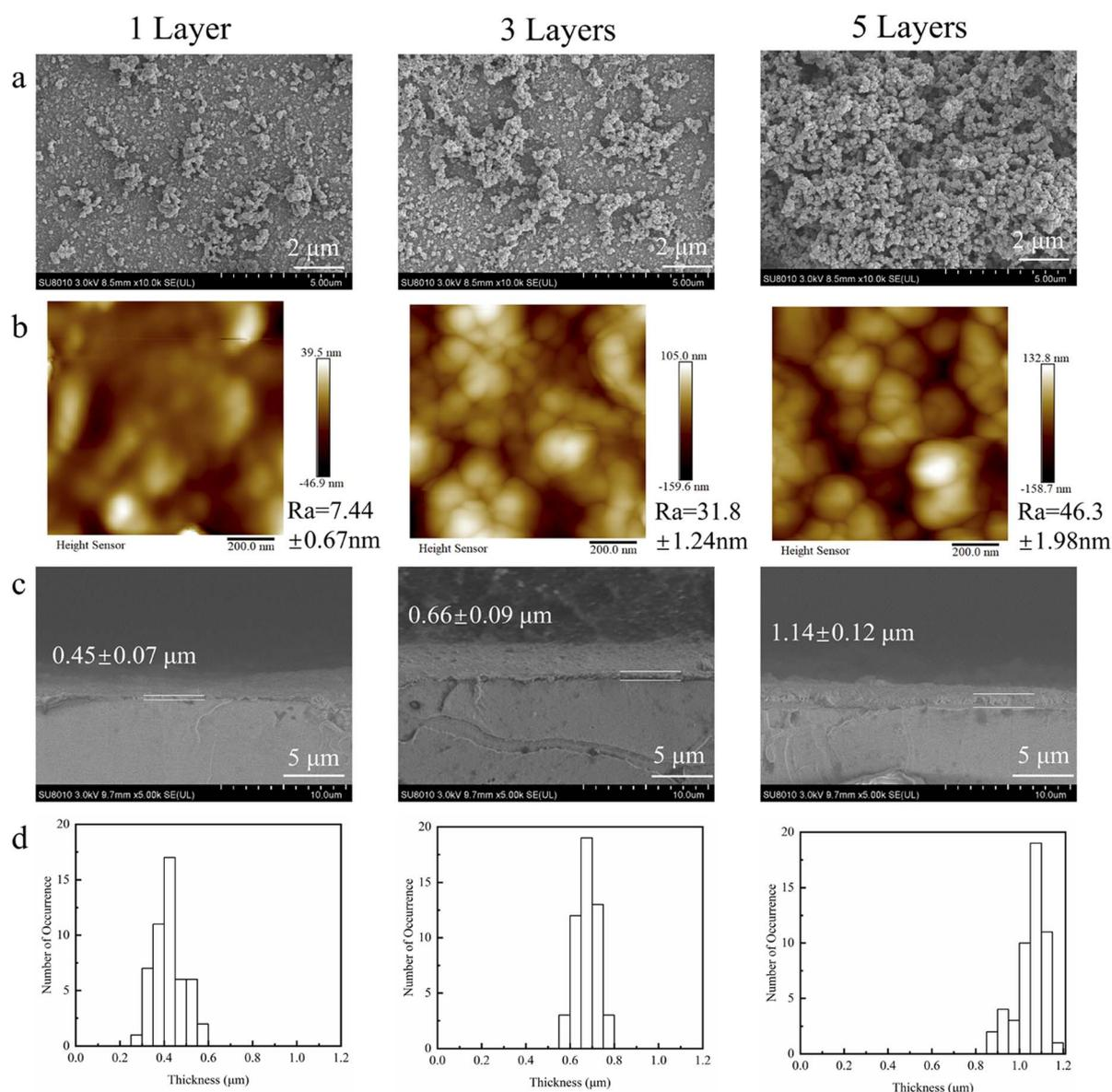
Fig. 2 Surface SEM images (a); AFM surface topography images (b); cross-sectional SEM images (c); TA-Fe<sup>3+</sup> complex film thickness distribution (d) of TA-Fe<sup>3+</sup>/PET by two-pot process: 1 layer; 3 layers; 5 layers, respectively.
