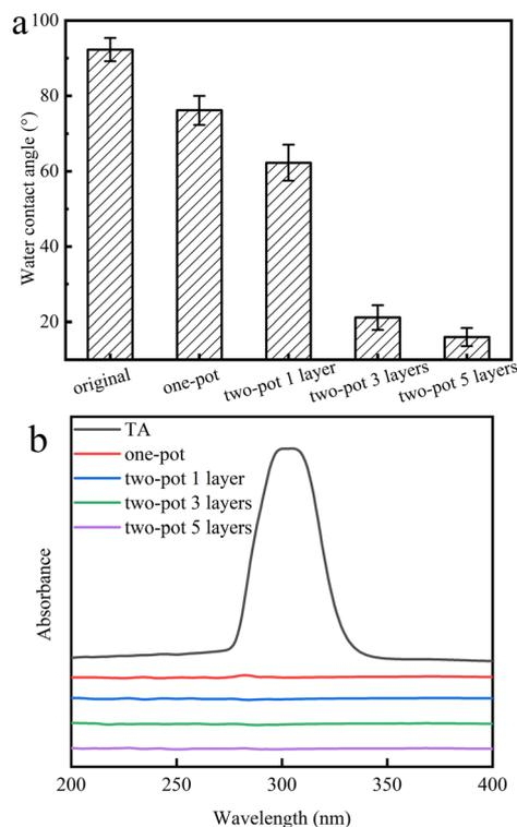
Fig. 3 Water contact angle of TA-Fe<sup>3+</sup>/PET (a); absorbance of solution after ultrasonic treatment of TA-Fe<sup>3+</sup>/PET, the control group: a 0.4 mg mL<sup>-1</sup> TA aqueous solution (b).
