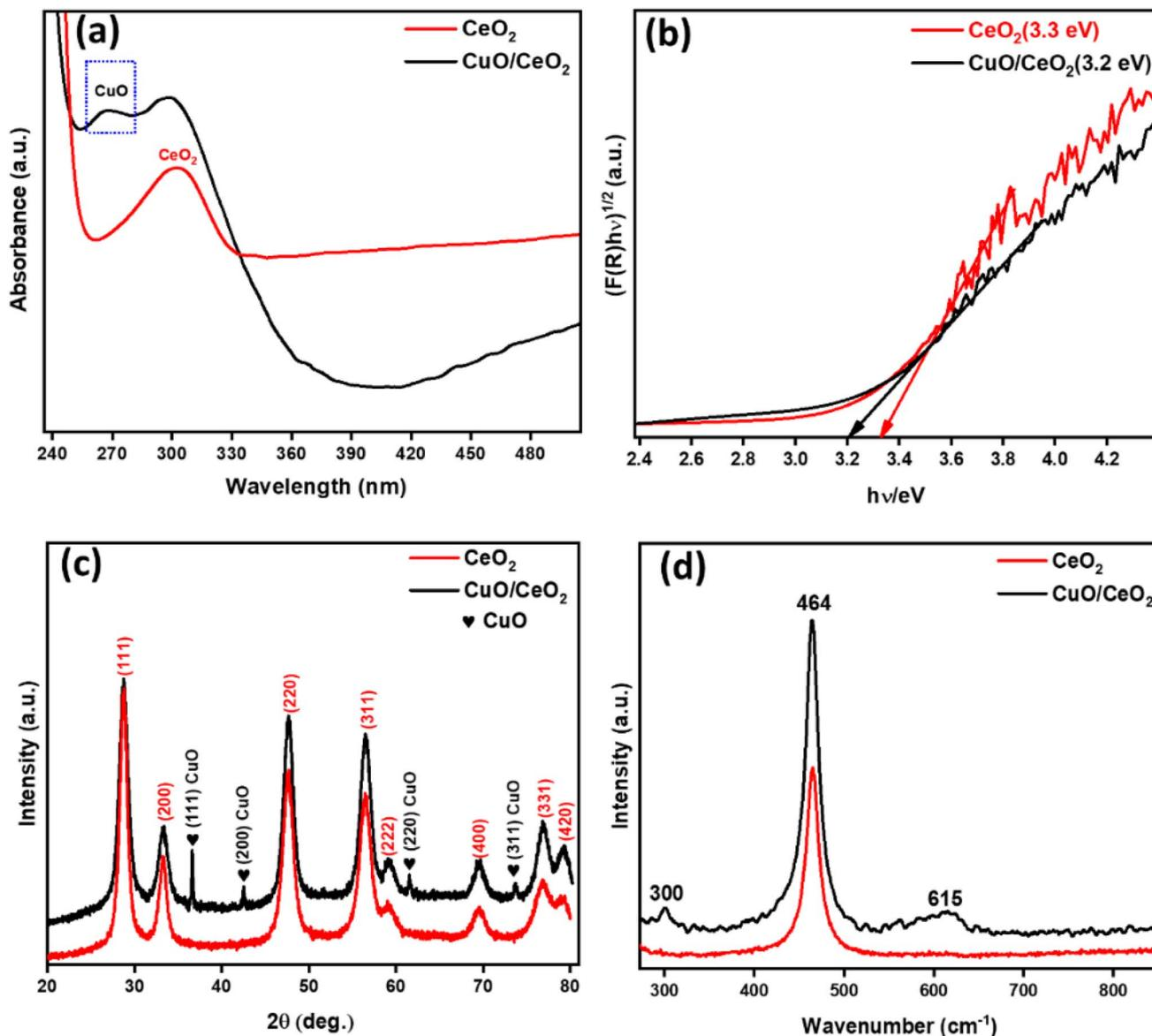
Fig. 1 Characterization results of CeO<sub>2</sub> and CuO/CeO<sub>2</sub> nanocomposites: (a) UV-vis absorption spectra, (b) band gap energy estimation using UV-vis diffuse reflectance spectroscopy (DRS) and the Kubelka–Munk (K–M) function, (c) powder X-ray diffraction (PXRD) patterns, revealing the crystalline structure and phase composition. (d) Raman spectra, providing insights into the vibrational properties and defect states of the materials.
