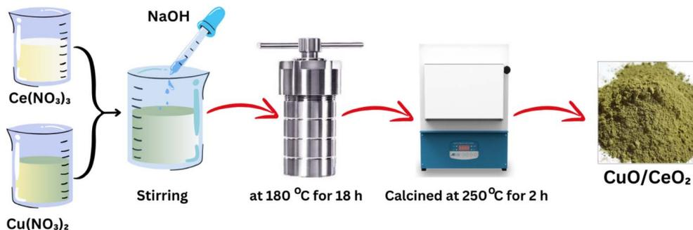
Scheme 1 Preparation of CuO/CeO<sub>2</sub> nanocomposites *via* the solvothermal method.
