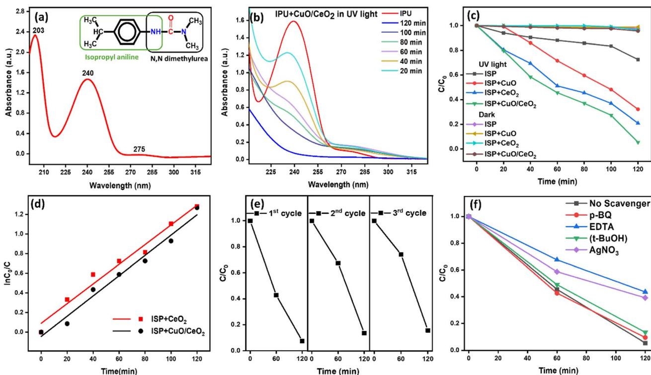
Fig. 5 (a) Structural formula and UV-vis spectra of isoproturon (b) UV absorption spectra of IPU with  $CuO/CeO_2$ , (c)  $C/C_0$  plot of IPU degradation, (d) kinetics of IPU degradation, (e) cyclic runs of the  $CuO/CeO_2$  nanocomposites and (f) photocatalytic activities of  $CuO/CeO_2$  with different scavengers for the degradation of IPU under UV light irradiation.
