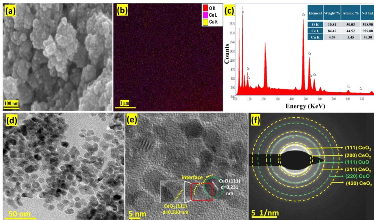
Fig. 3 (a) FESEM images of the CuO/CeO<sub>2</sub> nanocomposites, (b) overlay of Ce + O + Cu and (c) EDX spectra and the corresponding chemical composition analysis, (d) low-resolution TEM image, (e) HRTEM images with lattice fringes and (f) selected area electron diffraction (SAED) sequence of CuO/CeO<sub>2</sub> nanocomposites.
