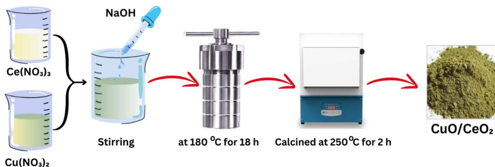
Scheme 1 Preparation of CuO/CeO 2 nanocomposites via the solvothermal method.
