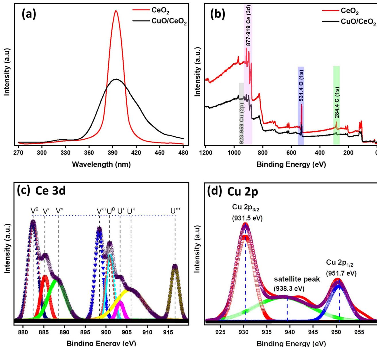
Fig. 2 (a) Photoluminescence spectra of CeO<sub>2</sub> and CuO/CeO<sub>2</sub> nanocomposites. XPS survey spectra of (b) CeO<sub>2</sub> and CuO/CeO<sub>2</sub> and deconvoluted spectra of (c) Ce 3d and (d) Cu 2p.
