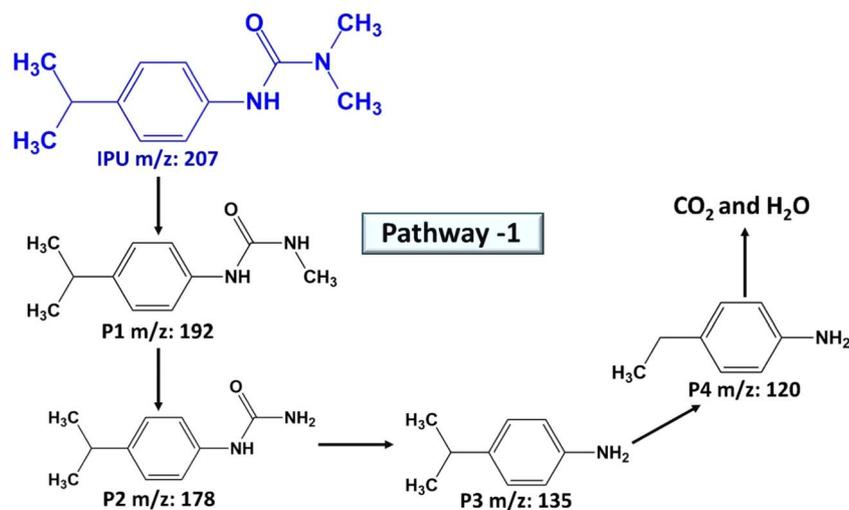
Fig. 7 IPU degradation intermediates detected using HRMS analysis.
