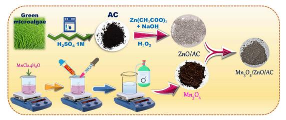
Scheme 1 The synthesis procedure of Mn<sub>3</sub>O<sub>4</sub>/ZnO/AG composite.
