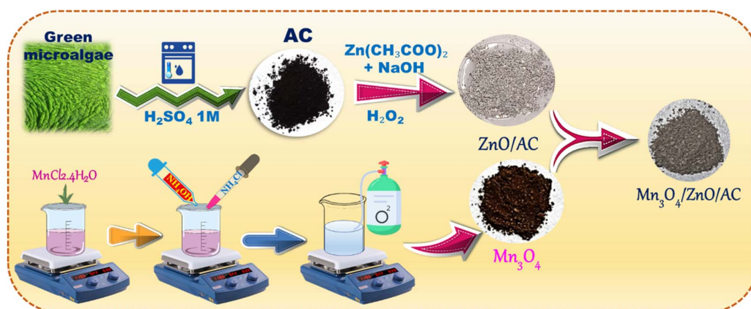
Scheme 1 The synthesis procedure of \text{Mn}_3\text{O}_4/\text{ZnO}/\text{AC} composite.
