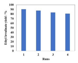
Fig. 2 Reusability of montmorillonite K10 for the esterification of levulinic acid with ethanol. Reaction conditions: montmorillonite K10, 100 mg; n-dodecane, 0.60 mmol; levulinic acid, 2.0 mmol; ethanol, 3.0 mL; temperature, 443 K; time, 3.75 h.
