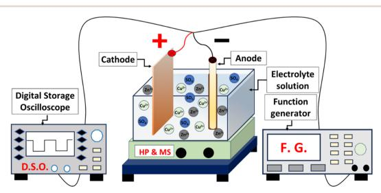
Fig. 1 Schematic of pulse electrodeposition experimental setup for Cu–Zn deposition.
