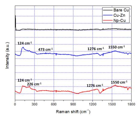
Fig. 13 Raman spectra obtained of bare Cu, electrodeposited Cu-Zn, and PC electrodes
