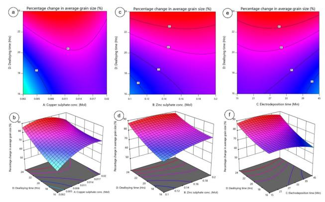
Fig. 5 2D contour and 3D plots for change in average grain size as a function of Cu, Zn sulphate concentration, electrodeposition time, and dealloying time.
