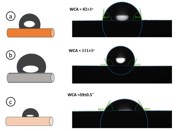
Fig. 15 Water contact angle of (a) bare Cu, (b) Cu-Zn, (c) NP-Cu electrodes.
