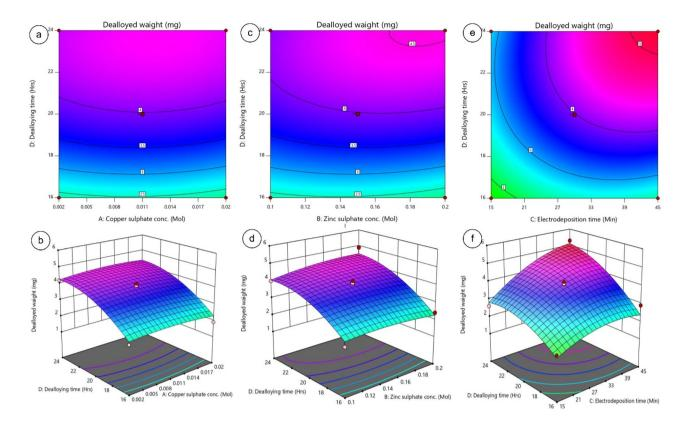
Fig. 4 2D contour and 3D plots for dealloyed weight as a function of Cu, Zn sulphate concentration, electrodeposition time, and dealloying time.
