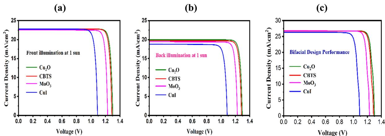
Fig. 14 Investigation of  $J$ - $V$  curves for the FTO/ZnO/Sr<sub>3</sub>PCL<sub>3</sub>/(Cu<sub>2</sub>O/CBTS/MoO<sub>3</sub>/CuI)/Ni device structure with (a) both front and (b) back illumination under 1 sun conditions and (c) a bifacial configuration.
