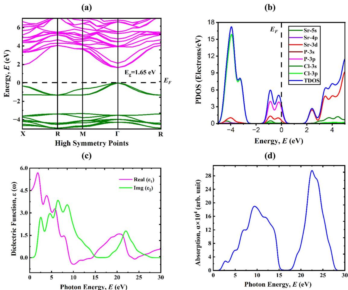
Fig. 2 An analysis of the  $\text{Sr}_3\text{PbCl}_3$  perovskite's (a) band structure, (b) PDOS, (c) dielectric function, and (d) absorption coefficient as functions of photon energy.
