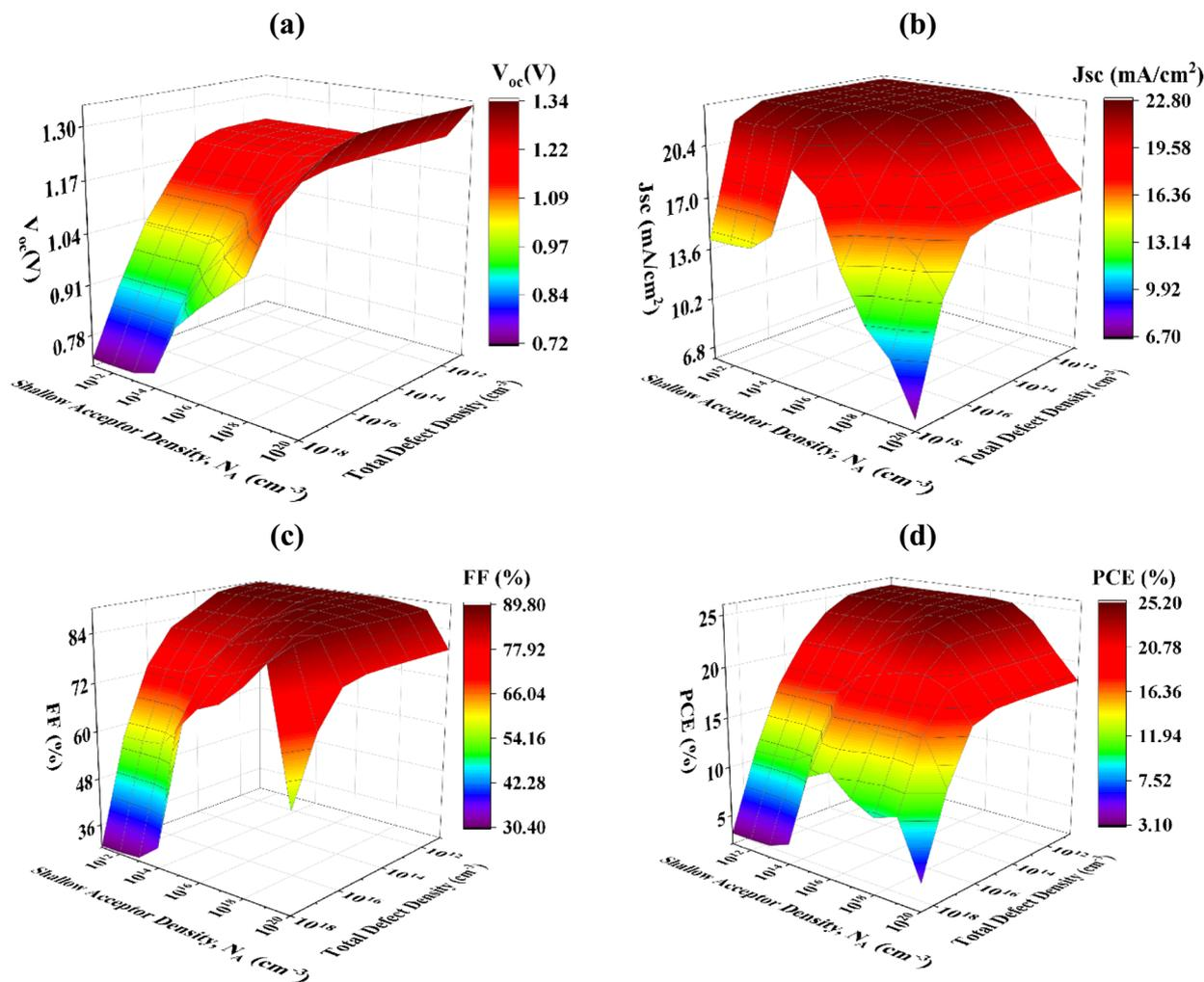
Fig. 7 Impact of  $\text{Sr}_3\text{PCL}_3$  absorber acceptor and bulk defect density variations on PV performance ((a)  $V_{\text{OC}}$ , (b)  $J_{\text{SC}}$ , (c) FF, and (d) PCE) with  $\text{MoO}_3$  HTL.
