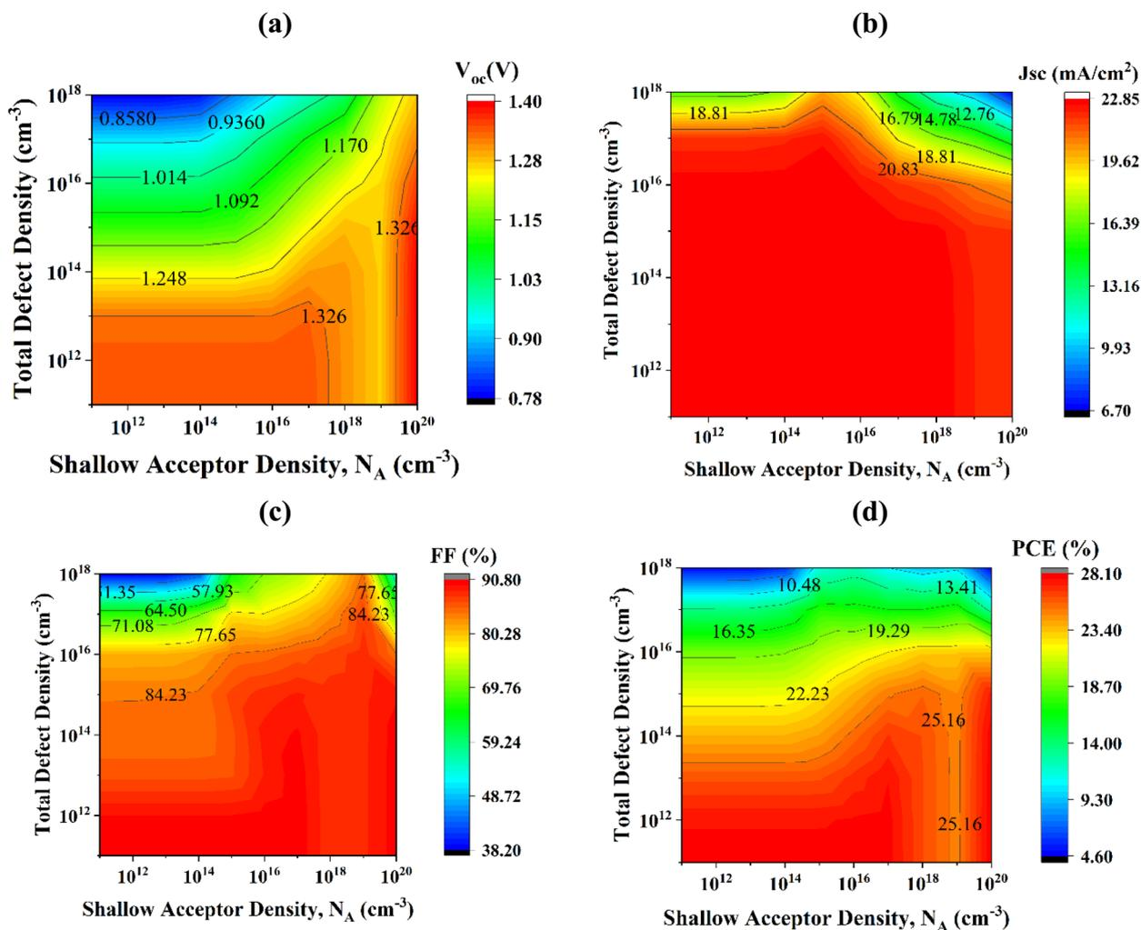
Fig. 5 Impact of Sr<sub>3</sub>PCl<sub>3</sub> absorber acceptor and bulk defect density variations on PV performance ((a)  $V_{OC}$ , (b)  $J_{SC}$ , (c) FF, and (d) PCE) with Cu<sub>2</sub>O HTL.
