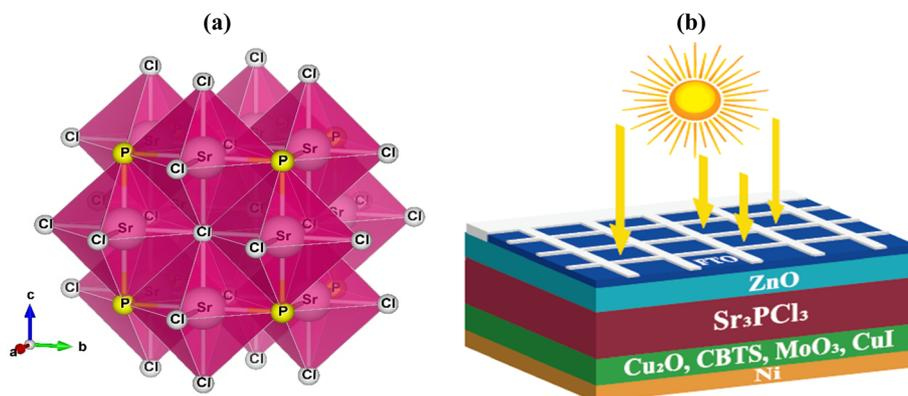
Fig. 1 The (a) crystalline configuration and (b) solar cell architecture of  $\text{Sr}_3\text{PCl}_3$  perovskite.
