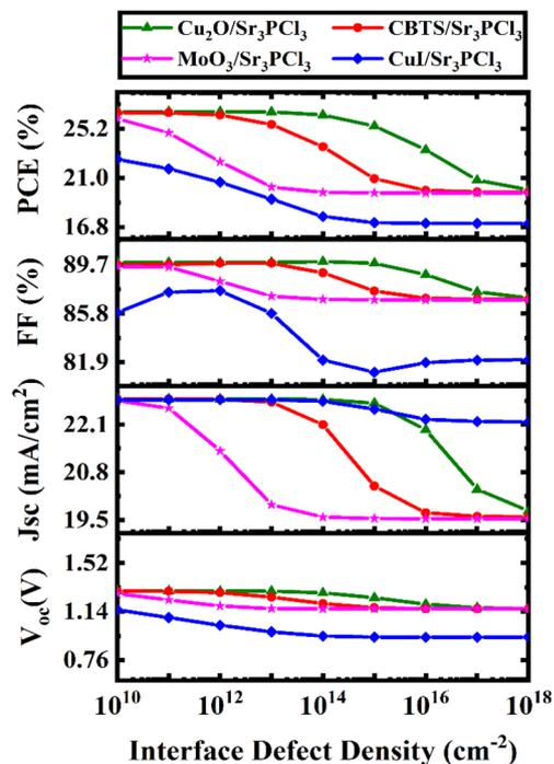
Fig. 10 Influence of variations in  $N_{\text{tf}}$  at various HTL/ $\text{Sr}_3\text{PbCl}_3$  layers on PV performance.
