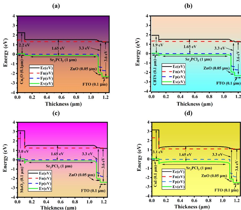
Fig. 3 EBD of the proposed four-device structure configurations (FTO/ZnO/Sr<sub>3</sub>PCL<sub>3</sub>/HTL/Ni) with different HTLs: (a) Cu<sub>2</sub>O, (b) CBTS, (c) MoO<sub>3</sub>, and (d) CuI.
