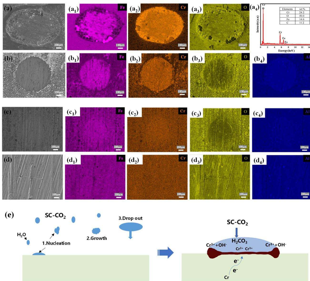
Fig. 5 SEM-EDS mappings of localized corrosion areas in Fe-5Cr-(0–3)Al alloy steels: (a–a<sub>4</sub>) 5Cr; (b–b<sub>4</sub>) 5Cr1Al; (c–c<sub>4</sub>) 5Cr2Al; (d–d<sub>4</sub>) 5Cr3Al, and localized corrosion mechanism diagram (e).
