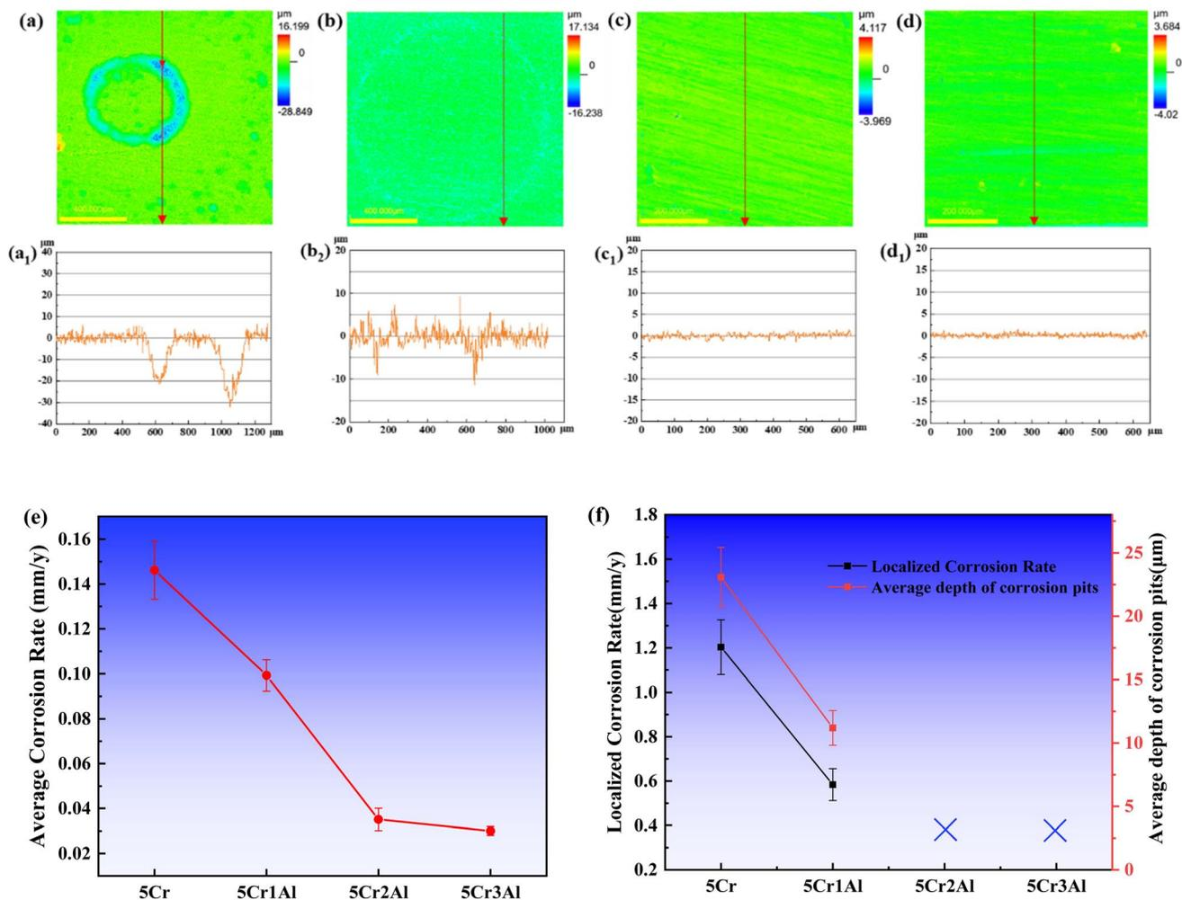
Fig. 3 Surface morphologies and linear profiles of Fe-5Cr-(0–3)Al alloys after removal of corrosion products: (a) and (a<sub>1</sub>) 5Cr; (b) and (b<sub>1</sub>) 5Cr1Al; (c) and (c<sub>1</sub>) 5Cr2Al; (d) and (d<sub>1</sub>) 5Cr3Al. (e) Presents the average corrosion rates and (f) shows the localized corrosion rates and average pit depths.
