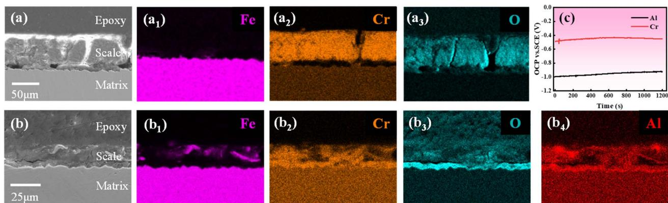
Fig. 6 SEM-EDS cross-sectional analysis of corrosion product layers in free water under sc-CO<sub>2</sub> environment. (a–a<sub>3</sub>) 5Cr; (b–b<sub>4</sub>) 5Cr2Al. (c) Open-circuit potential monitoring results of Cr and Al metals.
