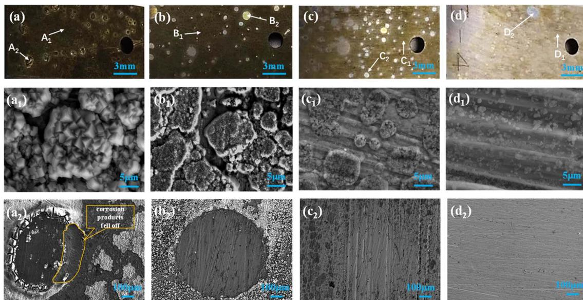
Fig. 2 (a) 5Cr, (b) 5Cr1Al, (c) 5Cr2Al, and (d) 5Cr3Al show the macroscopic morphologies of the alloys after corrosion. Corresponding SEM images of regions (A<sub>1</sub>–D<sub>1</sub>) are shown in (a<sub>1</sub>–d<sub>1</sub>), and SEM images of regions (A<sub>2</sub>–D<sub>2</sub>) are presented in (a<sub>2</sub>–d<sub>2</sub>).
