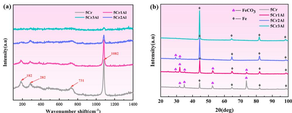
Fig. 4 Raman spectrum (a) and XRD spectrum (b) of the surface corrosion product film of Fe-5Cr-(0–3)Al alloy steels after 168 hours of immersion in water-saturated sc-CO<sub>2</sub> phase.
