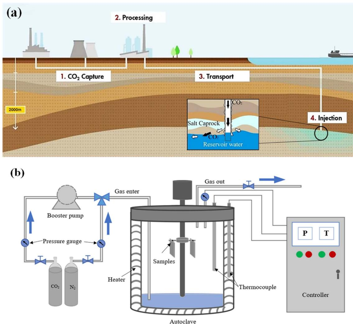
Fig. 1 Diagram showing an example of the CCUS process: modified from <https://Shell.com> (a)<sup>26</sup> and experimental setup for the high-pressure corrosion tests (b).
