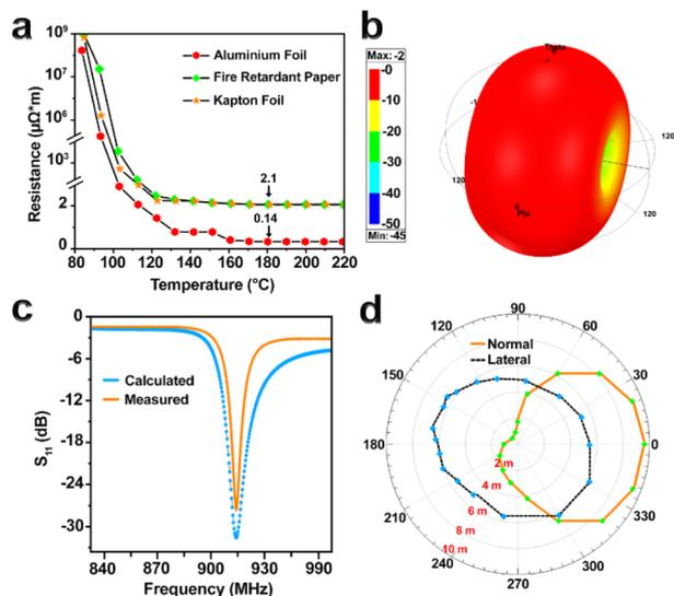
Fig. 3 (a) The graph displays the resistance values at different temperatures. (b) The three-dimensional radiation pattern of the UHF dipole RFID tag antenna model was calculated using HFSS. (c) The  $S_{11}$  results of the fabricated UHF dipole tag antennae were both calculated and measured. (d) The 915 MHz read range pattern of the antenna with an aluminum substrate was recorded, showing superior performance compared to non-metallic substrates (as depicted in ESI Table S3†).
