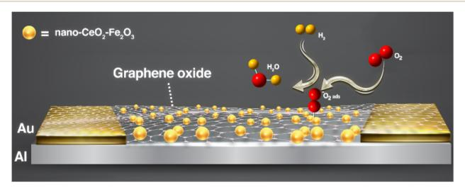
Fig. 8 The hydrogen gas sensing mechanism of nono- $CeO_2$ - $Fe_2O_3$ -GO is depicted in the schematic. When exposed to air, the sensor absorbs molecular oxygen and converts it into  $O_2$ . Upon exposure to hydrogen, the sensor facilitates the production of  $H_2O$ , resulting in a decrease in resistance.
