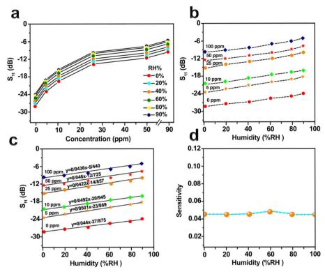
Fig. 7 (a) The  $S_{11}$  were obtained from various  $H_2$  concentrations at relative humidity levels ranging from 0% to 90% RH. (b) The  $S_{11}$  were obtained at  $H_2$  concentrations ranging from 0 to 100 ppm under relative humidity levels of 0% to 90% RH. (c) Utilizing linear regression to fit the  $S_{11}$  values. (d) Employing a quartic polynomial curve to fit the average humidity sensitivity.
