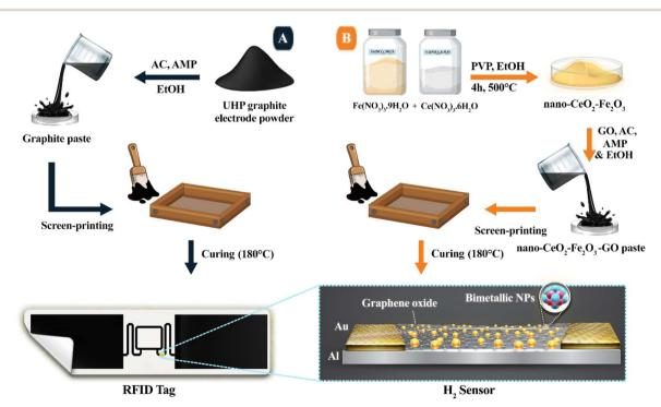
Fig. 1 (A) General scheme for graphite paste fabrication and RFID tag screen printing (B) fabrication of nano- $CeO_2-Fe_2O_3-GO$  and chemical resistance  $H_2$  sensing system with wireless detection.
