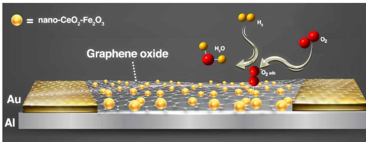
Fig. 8 The hydrogen gas sensing mechanism of nano- $CeO_2-Fe_2O_3-GO$  is depicted in the schematic. When exposed to air, the sensor absorbs molecular oxygen and converts it into  $O_2^-$ . Upon exposure to hydrogen, the sensor facilitates the production of  $H_2O$ , resulting in a decrease in resistance.
