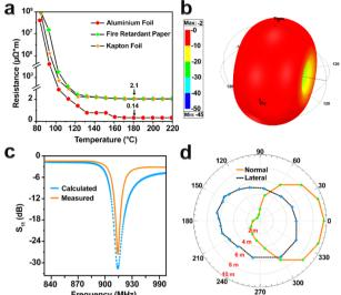
Fig. 3 (a) The graph displays the resistance values at different temperatures. (b) The three-dimensional radiation pattern of the UHF dipole RFID tag antenna model was calculated using HFSS. (c) The  $S_{11}$  results of the fabricated UHF dipole tag antennae were both calculated and measured. (d) The 915 MHz read range pattern of the antenna with an aluminum substrate was recorded, showing superior performance compared to non-metallic substrates (as depicted in ESI Table S3†).
