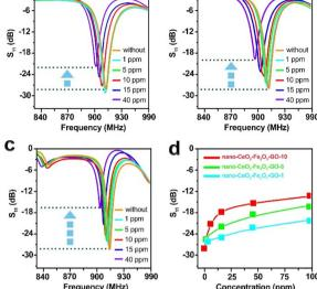
Fig. 6 Changes in the reflectance of sensors in different concentrations of hydrogen gas for (a) nono-CeO $_2$ -Fe $_2$ O $_3$ -GO-1. (b) Nono-CeO $_2$ -Fe $_2$ O $_3$ -GO-5. (c) Nono-CeO $_2$ -Fe $_2$ O $_3$ -GO-10. (d) Calibration curves for prepared sensors as a function of H $_2$  concentration, (red: nono-CeO $_2$ -Fe $_2$ O $_3$ -GO-10; green: nono-CeO $_2$ -Fe $_2$ O $_3$ -GO-5; cyan: nono-CeO $_2$ -Fe $_2$ O $_3$ -GO-1).
