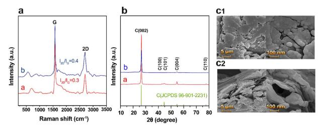
Fig. 2 Effects of treatment on UHP-GE. (a) Raman spectrum of UHP-GE (a), Raman spectrum of UHP-GE paste after treatment and curing at 180 °C (b). (b) XRD patterns of UHP-GE before (a) and after (b) treatment. (c1) FESEM images of UHP-GE before treatment and (c2) after.
