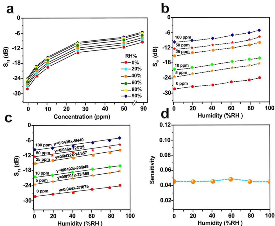
Fig. 7 (a) The  $S_{11}$  were obtained from various  $H_2$  concentrations at relative humidity levels ranging from 0% to 90% RH. (b) The  $S_{11}$  were obtained at  $H_2$  concentrations ranging from 0 to 100 ppm under relative humidity levels of 0% to 90% RH. (c) Utilizing linear regression to fit the  $S_{11}$  values. (d) Employing a quartic polynomial curve to fit the average humidity sensitivity.
