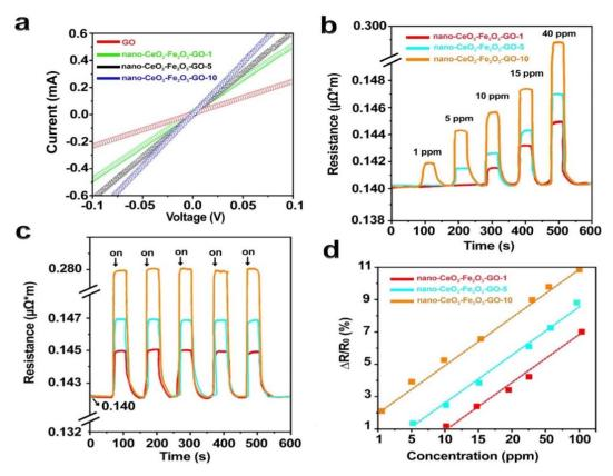
Fig. 5 (a) The current–voltage curves of the sensors, which were fabricated using nano- $CeO_2$ – $Fe_2O_3$  on the surface of graphene oxide, were measured with a current value ranging from 5 to 10 amperes. (b) The resistance was observed to change as a function of hydrogen gas concentration over time. (c) The sensors were exposed to 40 ppm hydrogen intermittently and periodically. (d) The nono- $CeO_2$ – $Fe_2O_3$ –GO sensor was calibrated for different concentrations of hydrogen gas.
