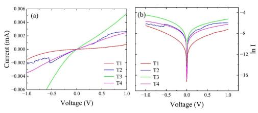
Fig. 7 (a) Linear and (b) semilog plots of the I-V characteristics of antimony sulfide films.
