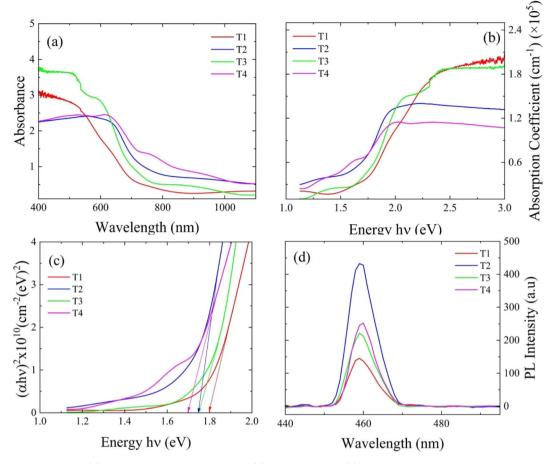
Fig. 6 (a) Absorbance spectra, (b) absorption coefficient spectra, (c) Tauc plots, and (d) photoluminescence spectra of antimony sulfide films.
