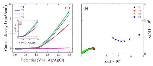
Fig. 8 (a) Cyclic voltammograms and (b) Nyquist plots of deposited antimony sulfide films.
