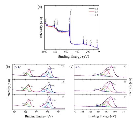
ig. 5 (a) Survey spectra, (b) & (c) core spectra of Sb 3d and S 2p of the antimony sulfide film.
