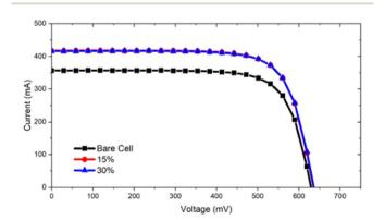
Fig. 3 I-V curves obtained under the irradiation of standard AM1.5G cells with LDSLs containing different concentrations of Eu(1DPIQC)<sub>3</sub> in PVB.
