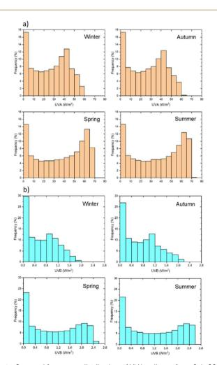
Fig. 1 Seasonal frequency distribution of UV irradiance from July 2023 to July 2024. (a) UV-A irradiance, and (b) UV-B irradiance.
