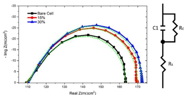
**Fig. 5** Nyquist plot under illumination conditions (under irradiation of standard AM1.5G) of  $\text{Eu}(\text{}^1\text{DPIQC})_3/\text{PVB}$  and bare c-Si cell. Green dotted curves represent the fit of the experimental curves.
