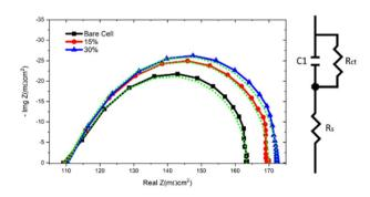
Fig. 5 Nyquist plot under illumination conditions (under irradiation of standard AM1.5G) of Eu(<sup>1</sup>DPIQC)<sub>3</sub>/PVB and bare c-Si cell. Green dotted curves represent the fit of the experimental curves.
