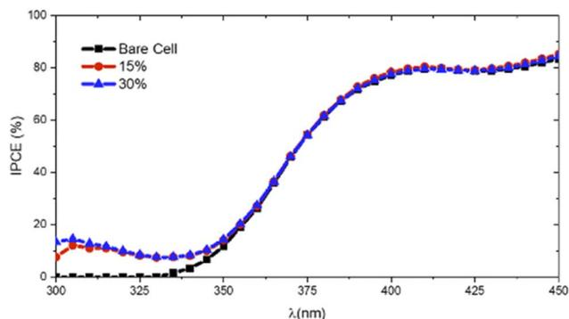
**Fig. 4** IPCE curves of a c-Si with LDSLs containing different concentrations of  $\text{Eu}(\text{}^1\text{DPIQC})_3/\text{PVB}$ .**Table 2** EQE values for some  $\text{Eu}^{3+}$ -based luminescent downshifting coatings<sup>a</sup>
