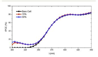
Fig. 4 IPCE curves of a c-Si with LDSLs containing different concentrations of Eu(1DPIQC)3/PVB.
