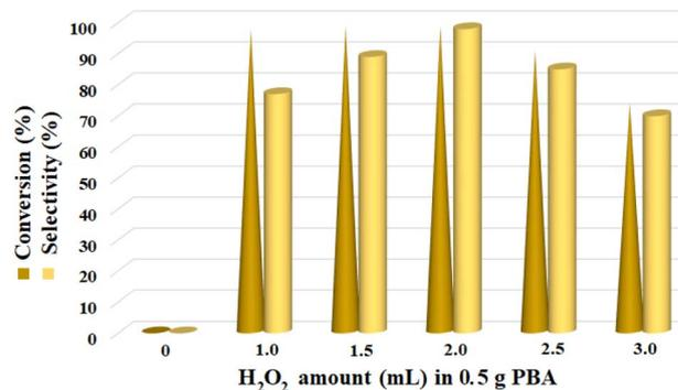
Fig. 1 Screening of H<sub>2</sub>O<sub>2</sub> : PBA (PSA amount was considered constant as 0.5 g) ratio over the epoxidation reaction of styrene at 0 °C for 4 h.
