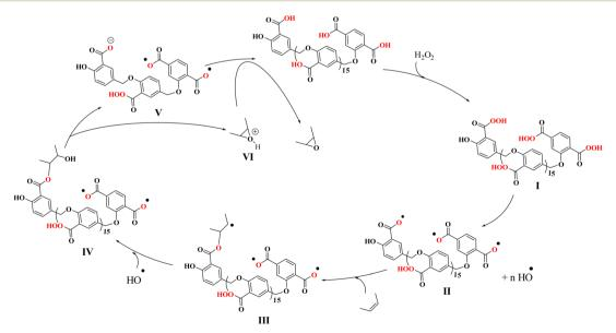
Scheme 5 A proposed mechanism for the radical transformation of olefin to epoxide catalyzed by PBA/H<sub>2</sub>O<sub>2</sub> system.
