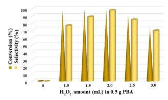
Fig. 1 Screening of  $H_2O_2$ : PBA (PSA amount was considered constant as 0.5 g) ratio over the epoxidation reaction of styrene at 0 °C for 4 h.
