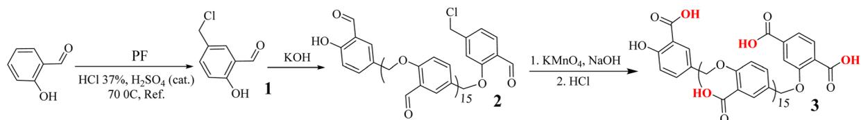
Scheme 1 Synthesis of PSA and PBA.<sup>23</sup>
