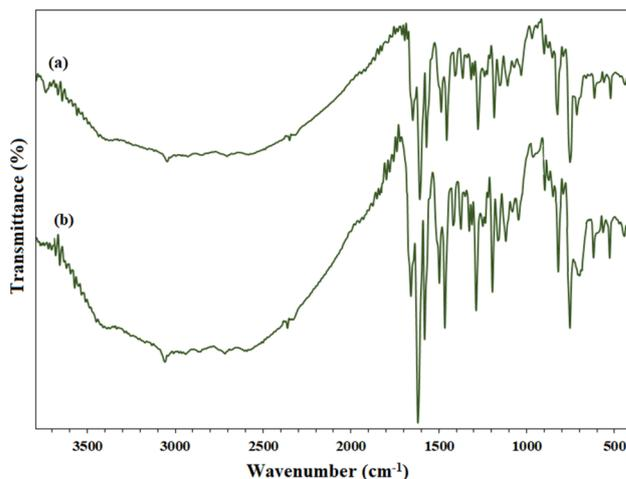
Fig. 4 FTIR spectrum of the (a) freshly prepared PBA<sup>30</sup> and (b) recycled PBA after 7th recycle in the reaction of benzyl alcohol to benzoic acid at ambient temperature.
