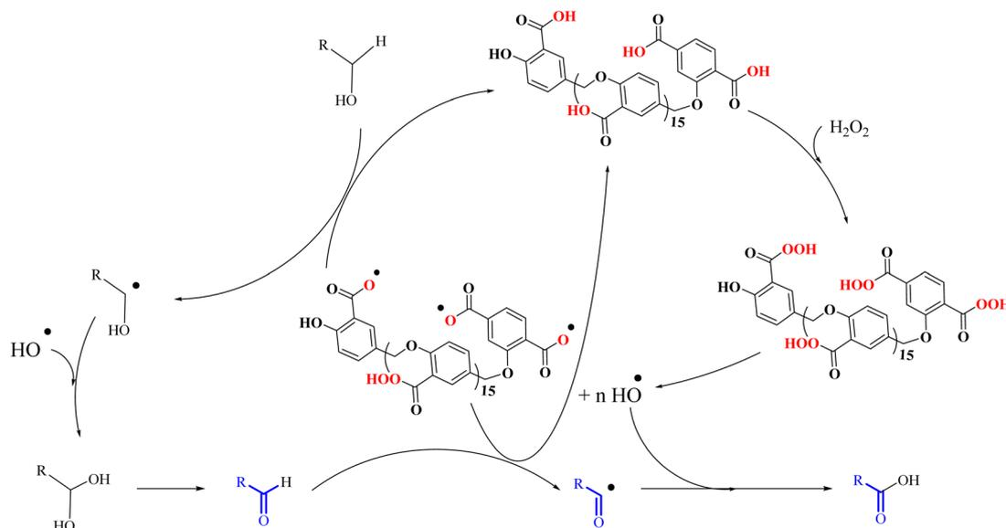
Scheme 4 A plausible mechanism for direct oxidation of alcohols to benzoic acid by PBA in H<sub>2</sub>O<sub>2</sub> in water at ambient temperature—a radical mechanism.
