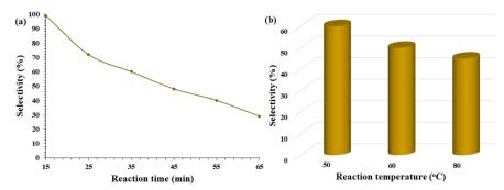
Fig. 2 Selectivity monitoring over the epoxidation of styrene towards (a) reaction time after 15 min in an ice bath and (b) in different reaction temperature.
