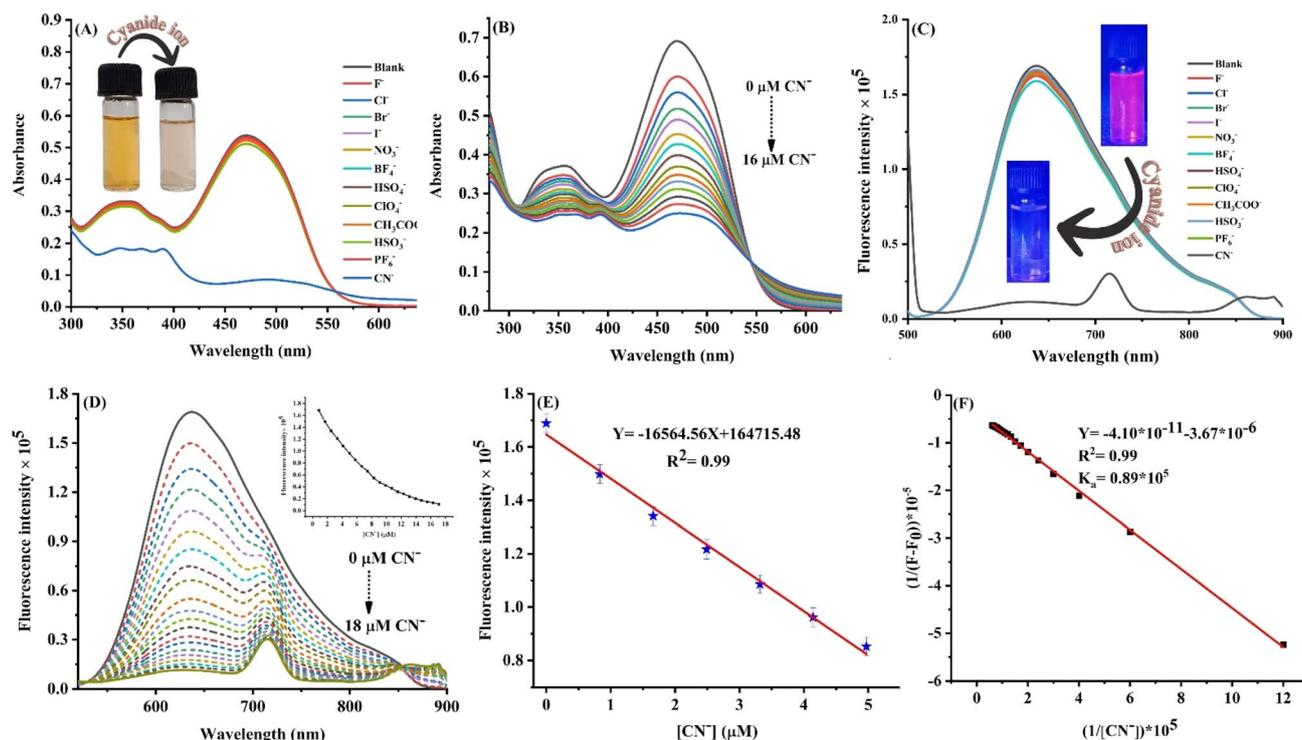
Fig. 3 (A) Absorption spectra of the probe in the presence of different anions; (B) titration profile of ADTI with increasing concentration of cyanide ion (0–16  $\mu\text{M}$ ); (C) emission spectra of probe in the presence of various anions; (D) influence of cyanide concentration on the emission spectra of the probe; (E) LOD plot; and (F) Benesi–Hildebrand plot.
