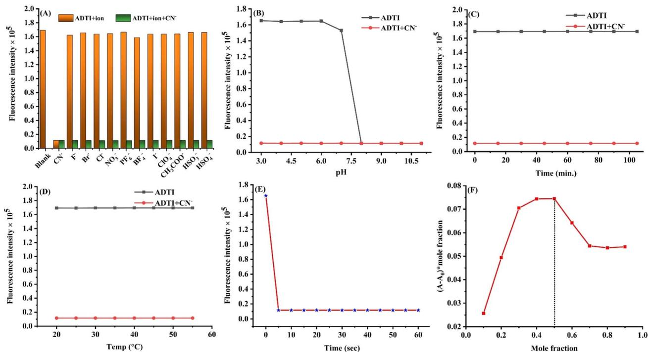
Fig. 4 (A) Interference studies in the presence of other ion; (B) effect of pH on ADTI and "ADTI-CN<sup>-</sup>" adduct (C) response time; (D) photostability of ADTI and "ADTI-CN<sup>-</sup>" adduct; (E) thermal stability of ADTI and "ADTI-CN<sup>-</sup>" adduct; (F) Job's plot.
