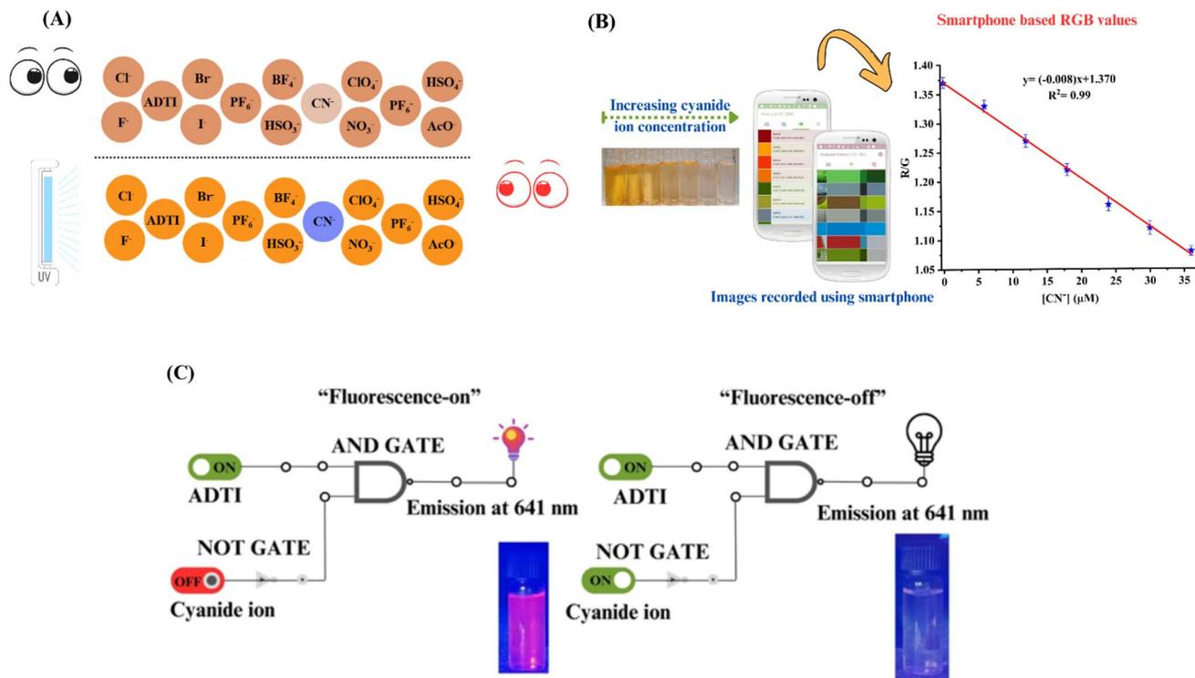
Fig. 6 (A) Filter paper based test strip for cyanide detection under naked eye and UV-lamp; (B) smartphone based sensing of CN<sup>-</sup> in aqueous solution of sensor ADTI; (C) INHIBIT logic gate.
