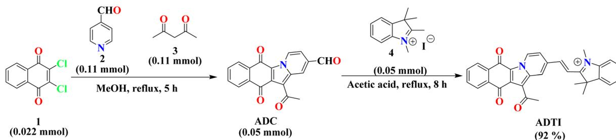
Scheme 1 Acetic acid catalysed synthesis of probe (ADTI).
