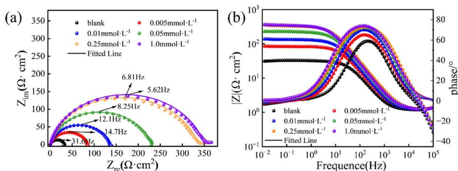
Fig. 4 Nyquist (a) and Bode-phase angle plots (b) for Q235 CS in 1.0 mol per L HCl containing different concentrations of PBT at 298.15 K.
