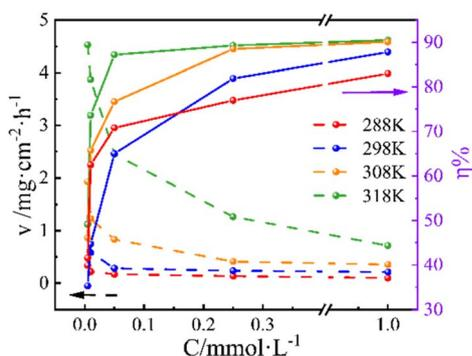
Fig. 1 Variation of corrosion rate ( $v$ ) and inhibition efficiency ( $\eta$ ) with concentrations of PBT in 1.0 mol per L HCl at different temperatures. Noted that means and standard deviations were obtained from triplicate samples at least, where error bars that lie within the data points themselves are not visible.
