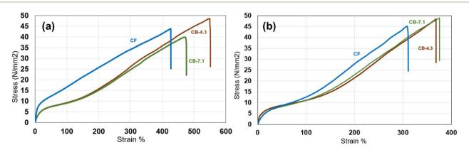
Fig. 4 Stress-strain curves for CF and CB samples: (a) films produced by melt compression molding, and (b) films cast from solution. Only the CF film from compression molding exhibits significantly different behavior, characterized by a distinct elastic region followed by a linear strain-hardening region. The tensile behavior of CB 4.3 and 7.1 are similar.
