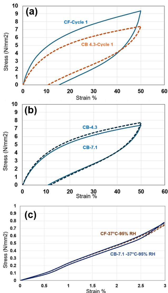
**Fig. 5** Hysteresis Stress–Strain curve for samples cast from solution (a) CF and CB 4.3 with CF showing a higher stress but smaller strain recovery, (b) two CBs 4.3 and 7.1 show very similar behavior indicating the insignificant effect of molecular weight, (c) Curve for CF and CB 7.1 at 37 °C and 95% RH in the elastic region (3% strain) where the behavior of two polymers are very similar.
