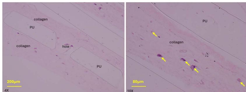
Fig. 8 Cross section images of H&E-stained CF mesh at 4× magnification (left) and 10× magnification (right). A uniform sheet of collagen gel matrix with small numbers of individual cells scattered through the matrix was formed on top, bottom, and through the hole of the CF mesh. Yellow arrows: cells.
