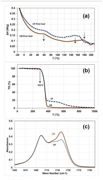
Fig. 6 (a) DSC results first heat for CF and CB 7.1 displays minimal peaks where thermal transition peaks are not significant for this type of polymers (b) TGA results for casted CF and CB, CF shows two step behavior change with 80% of the mass loss occurring in the first step, (c) FTIR spectrum of CB 7.1 and CF films prepared from solution casting, two strong peaks at 1700 and 1735 cm $^{-1}$  are assigned to N–H-bonded C=O (C=O···N–H) and the free C=O stretching vibration, respectively.
