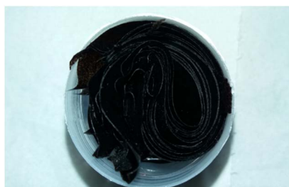
Fig. 5 Prepared GO-CMC-MMT-3 membrane type nanocomposite.
