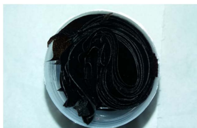
Fig. 5 Prepared GO-CMC-MMT-3 membrane type nanocomposite.
