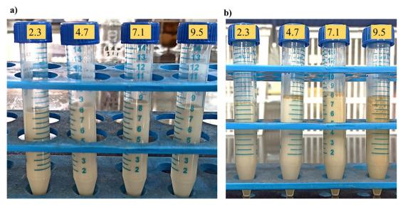
Fig. 3 NE formulations on the (a) 0<sup>th</sup> day showing no phase separation and (b) after 30 days showing little phase separation in NE with O/S of 4.7 and 51 and 51 and 51 and 51 and 51 and 51 and 52 and 51 and 52 a
