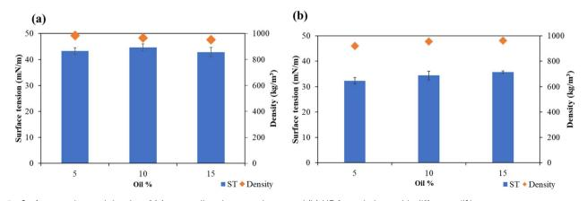
Fig. 5 Surface tension and density of (a) neem oil and water mixture and (b) NE formulations with different oil%.
