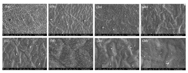
Fig. 6 SEM images of (1) rose and (2) hibiscus leaves as viewed under (a)  $500\times$ , (b)  $1000\times$ , (c)  $2000\times$ , and (d)  $5000\times$ .
