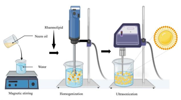
Fig. 1 Schematic of rhamnolipid stabilized neem oil NE synthesis.
