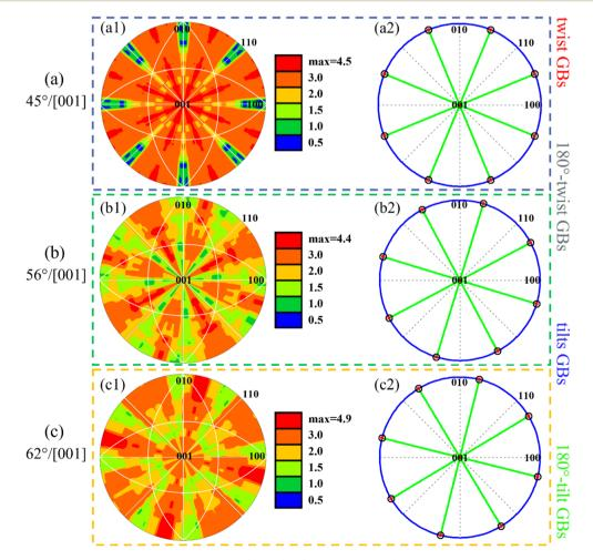
$\textbf{Fig. 6} \quad \textbf{Grain boundary plane orientation distribution function (GBP-ODF) maps of hot-deformed \ Nd_2Fe_{14}B \ permanent \ magnets \ and \ theoretical \ properties of the properties of$ geometrical feature positions, (a) 45°, (b) 56° and (c) 62°. Orientation texture intensity is given in MRD.
