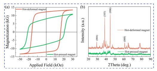
Fig. 2 Hysteresis loops (a) and XRD patterns (b) of Nd<sub>2</sub>Fe<sub>14</sub>B permanent magnet, perpendicular magnet surfaces were obtained.
