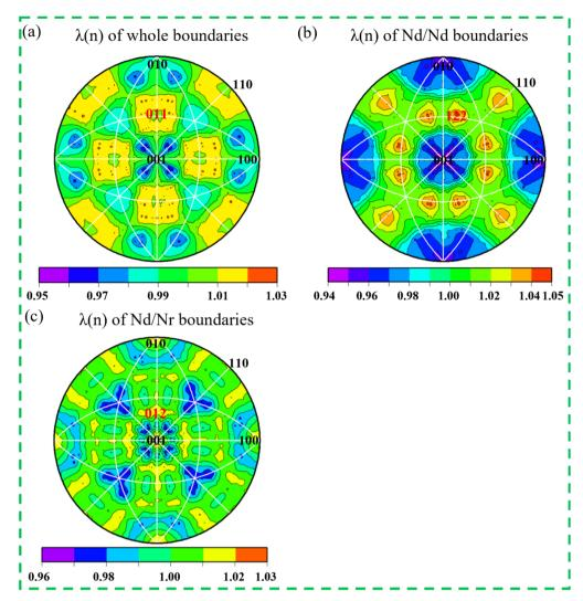
Fig. 7 Orientation distribution of  $\lambda(n)$  on the habit plane of hot-deformed Nd<sub>2</sub>Fe<sub>14</sub>B permanent magnets, (a) whole boundaries; (b) Nd/Nd grain boundaries; (c) Nd/Nr phase boundaries. Orientation texture intensity is given in MRD.
