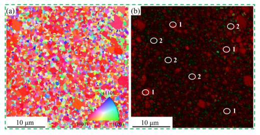
Fig. 3 Inverse pole figure quick map of microstructure in the measurement region of hot-deformed  $Nd_2Fe_{14}B$  permanent magnet (a), the phase map of the  $Nd_2Fe_{14}B$  permanent magnet imposed on the image quality map, with red color represent the main phase  $Nd_2Fe_{14}B$  and green color represent Nd-rich (b).
