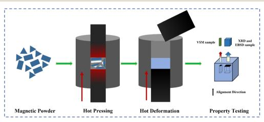
Fig. 1 Preparation process diagram of hot-deformed magnet.
