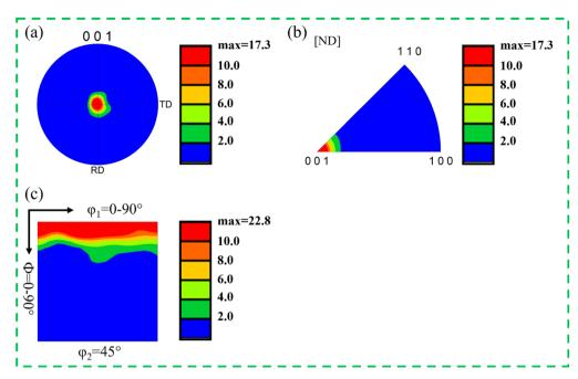
Fig. 4 Pole figure (a), inverse pole figure (b) and orientation distribution function (c) of the hot-deformed  $Nd_2Fe_{14}B$  permanent magnet. Orientation texture intensity is given in MRD.
