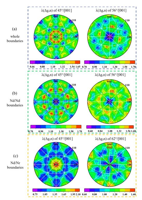
Fig. 8 Orientation distribution of  $\lambda(\Delta g, n)$  for hot-deformed Nd<sub>2</sub>Fe<sub>14</sub>B permanent magnets, (a) whole boundaries; (b) Nd/Nd grain boundaries; (c) Nd/Nr phase boundaries. Orientation texture intensity is given in MRD.
