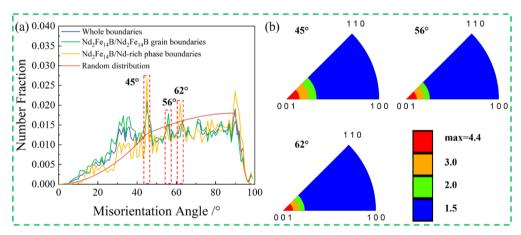
Fig. 5 Misorientation angle distribution of hot-deformed  $Nd_2Fe_{14}B$  permanent magnet(a) and axis/angle misorientation distribution functions for hot-deformed  $Nd_2Fe_{14}B$  magnet(b). Orientation texture intensity is given in MRD.
