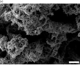
Fig. 3 SEM micrographs showing YBCO sponge. Scale bars are 100  $\mu m$  in (a) and 20  $\mu m$  in (b).
