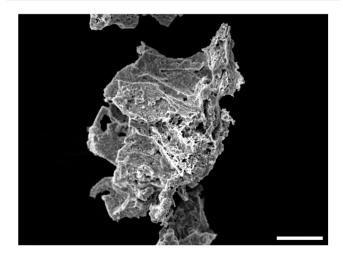
Fig. 4 SEM micrograph showing YBCO prepared without the use of templates. The scale bar is 20  $\mu m.\,$
