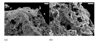
Fig. 8 SEM micrographs showing BSCCO sponges. Scale bar in (a) is  $100~\mu m$  and  $20~\mu m$  in (b).
