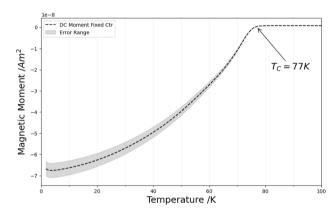
Fig. 11 SQUID magnetometry measurement of BSCCO.
