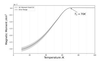
Fig. 7 SQUID magnetometry measurement of YBCO and BSCCO.
